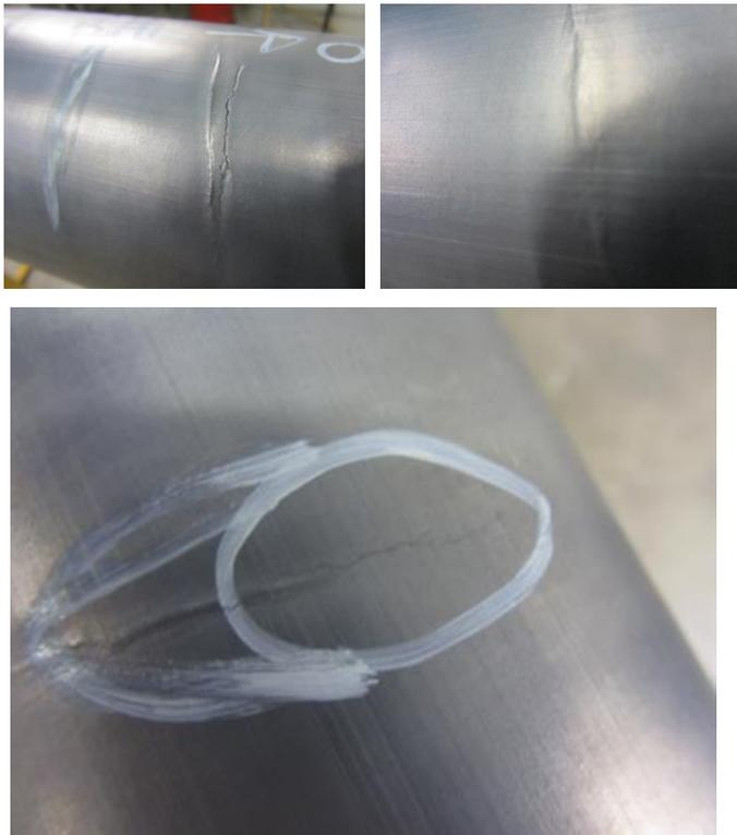
Fig. 9. (Upper Left) Outside of a (failed) XLPE power phase after 15,000 cycles at 1.1 %  $\Delta\epsilon$ ; (Upper Right) Outside of a (run- out) XLPE power phase after 25,000 cycles at 0.4 %  $\Delta\epsilon$ ; (Lower) Outside of a (failed) XLPE power phase after 30,000 cycles at 0.4 %  $\Delta\epsilon$ .
