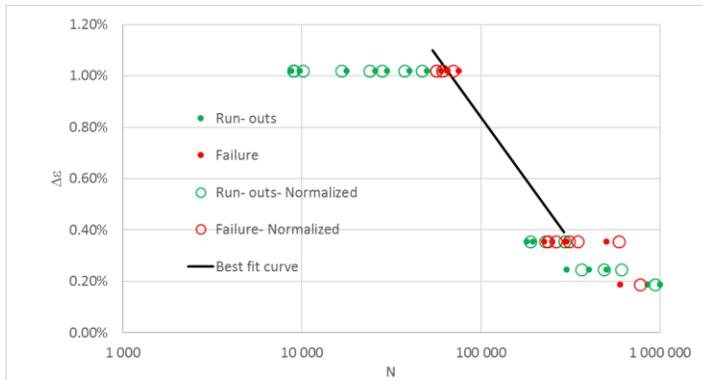
Fig. 5. Full scale results for MI power cables together with the results normalized to the average testing strain rate and the calculated maximum likelihood function.
