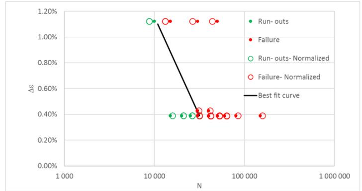
Fig. 6. Full scale results for XLPE power phases together with the results normalized to the average testing strain rate and calculated the maximum likelihood function.
