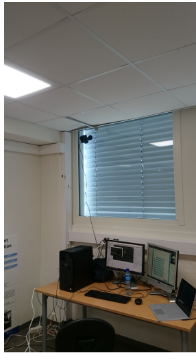
Figure 39: This image shows the alternative lighthouse setup that had to be made as the original ceiling mounted lighthouse disappeared before Experiment 2 started. Instead of a ceiling mounted solution, this setup makes use of a glass mounted lighthouse.
