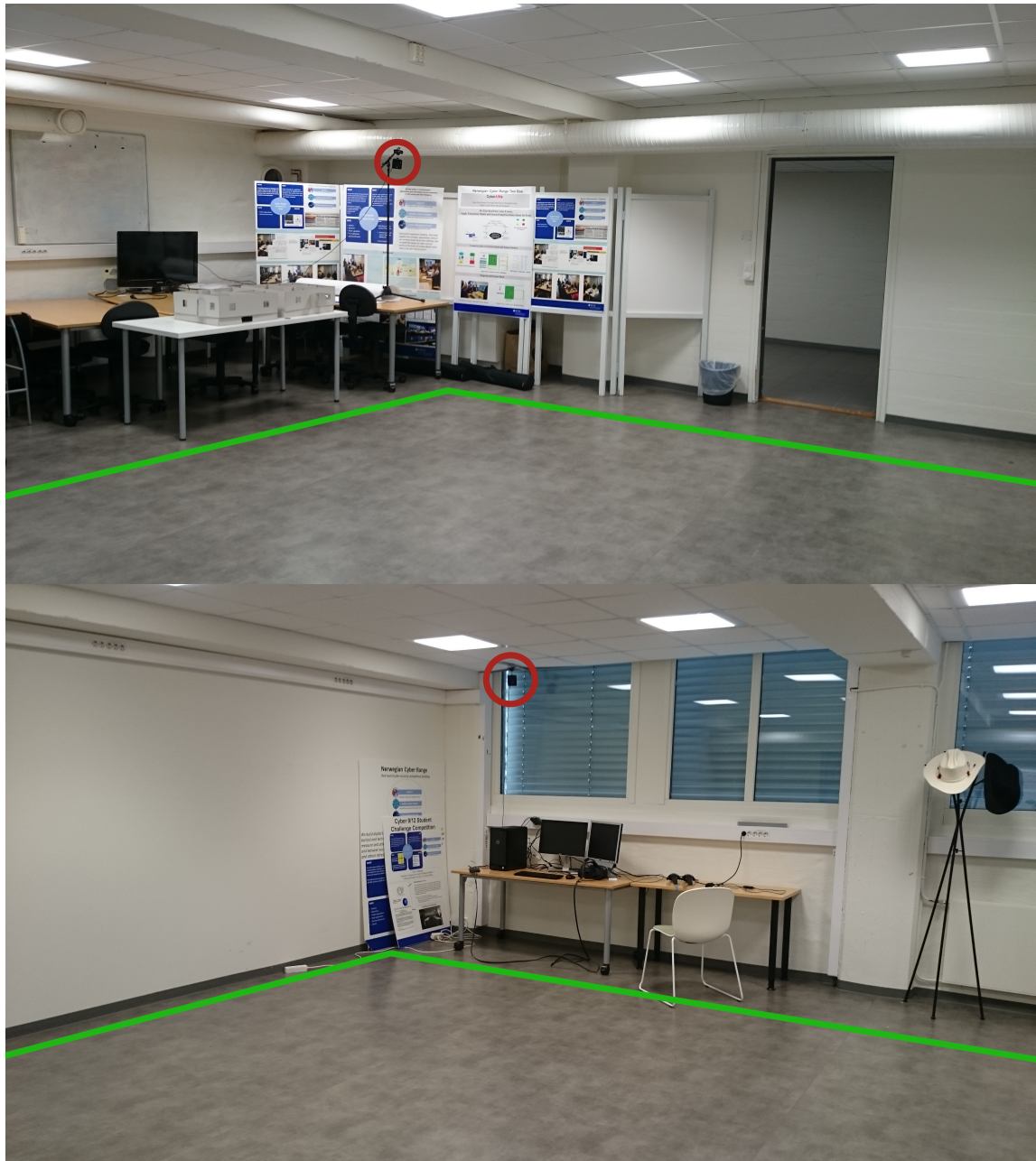
Figure 21: These two images show a rough outline of the physical tracking space that was used with green lines. Red circles are used to outline the location of the Vive Lighthouses.
