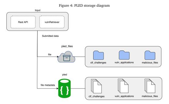
Figure [4] show how the different storage mechanisms are laid out. A file will be stored in the *pled\_files* container in Swift, and its metadata are added as a document in one of the three collections.
