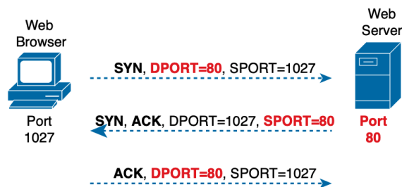
Figure 13: TCP connection establishment [53].
