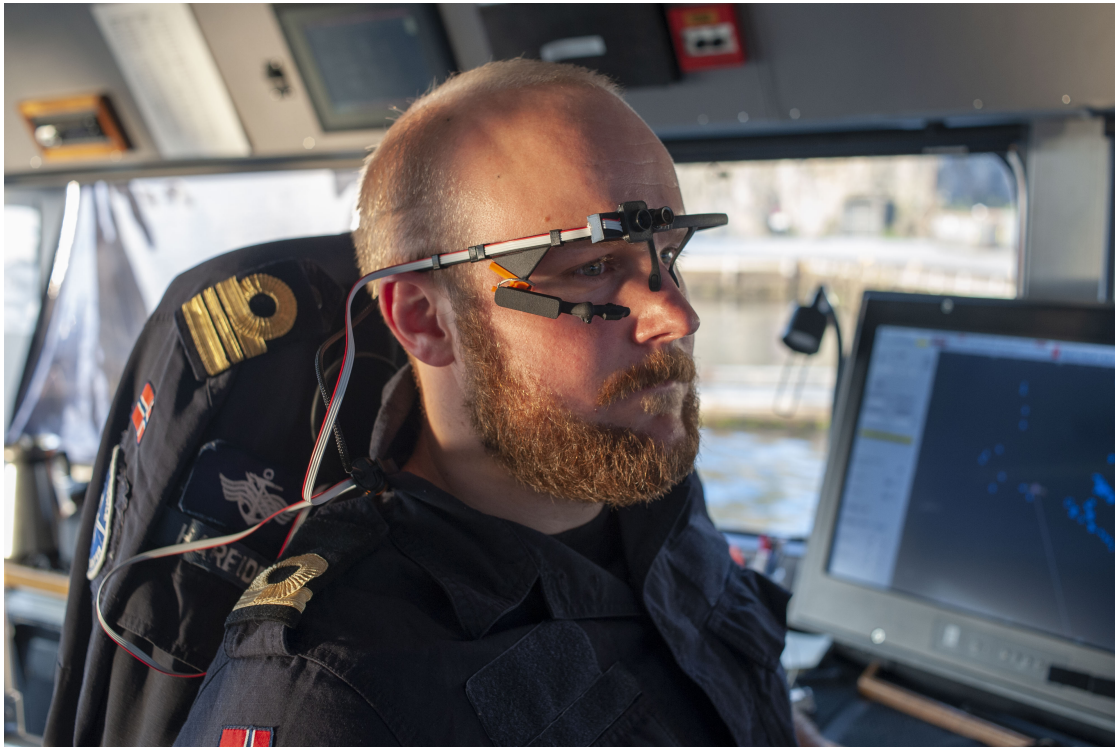
Figure 21: One of the study participants wearing the eye tracker and luminance sensor.
