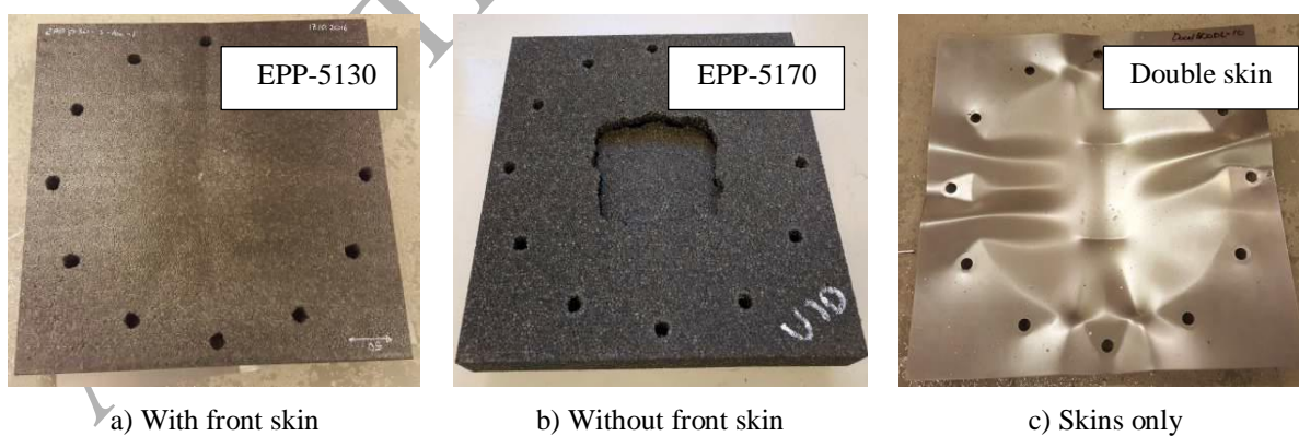
Figure 10. Pictures of typical EPP foam cores from a) configuration 1 and b) configuration 2, and c) picture of configuration 3, after an impact of 10 m/s.
