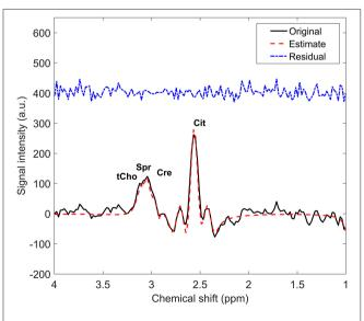
**FIGURE 1** | Example of a proton MR spectrum (solid line) of one voxel in healthy prostate tissue with the overlaid spectrum fit (red dash line) and the residuals (blue dash-dot line). tCho, total choline; Spr, spermine; Cre, creatine; Cit, citrate.
