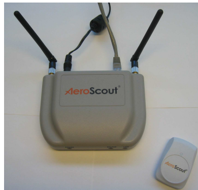
Figure B.4: Programming tags with the AeroScout Tag Activator
