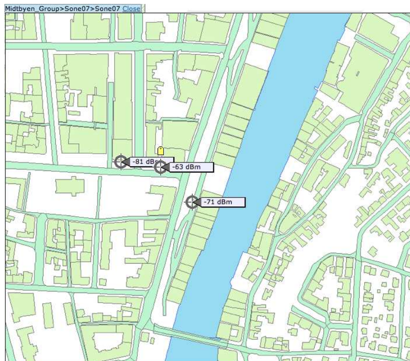
Figure 5.5: Tag monitoring in WCS. Detailed map with yellow marker indicating the tag location. The three surrounding access points that receive the tag messages, and the RSSI values they measure from the tag are also shown in this map.
