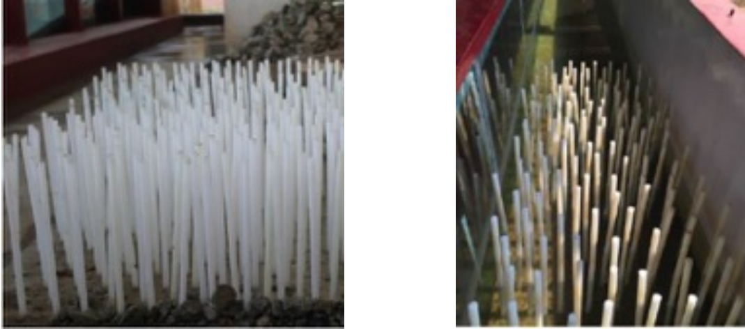
Figure 1: Experimental setup of emerged vegetation in wave flume [1]
