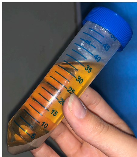
Figure 13. Tube after centrifugation of hydrolysate of HW (large-scale hydrolysis). Separated into sediment and hydrolysate fraction, but no oil fraction.
