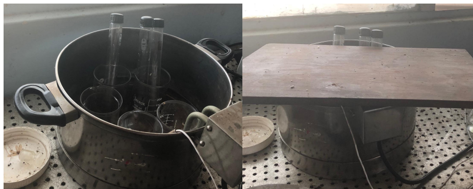
Figure 14. Setup of oil bath digestion to find L_{\max} when calculating % DH.
