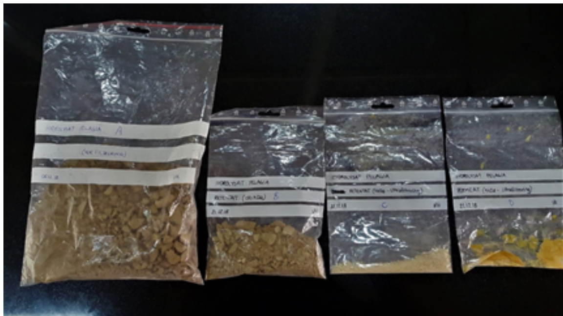
Figure 21. Freeze-dried hydrolysate from Pelagia, and the different fractions after fractionation by ultrafiltration (Brustad, 2019). From left: original hydrolysate, retentate >150 kDa, retentate >4 kDa and permeate <4 kDa.
