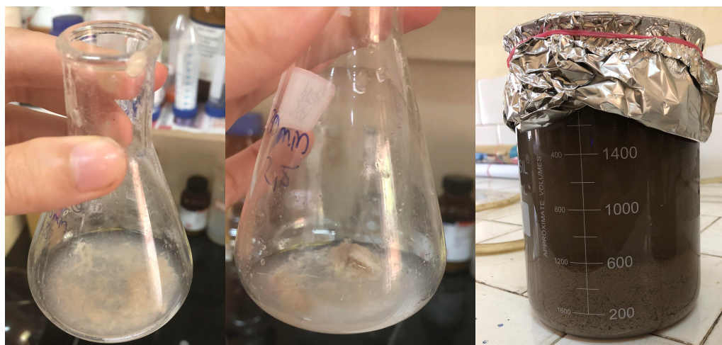
Figure 11. Illustration of the uneven distribution of raw material and water in the small-scale hydrolysis, as well as the large-scale hydrolysis of HW. The two conical flasks are from the small-scale hydrolysis of RW, where the flask on the right has a big chunk of raw material while the flask on the left is more homogenous. The big beaker was used for the large-scale hydrolysis of HW.
