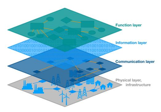
**Figure 2.3:** Illustration of the different layers that the smart grid consist of. Inspired by [70].
