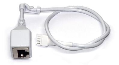
**Figure 3.4:** A 4-pin-to-RJ45 connector of this type will be inserted into the HAN port. The RJ45 contact will be outside the seal that is covering the smart meter. Photo: Aidon Ltd.
