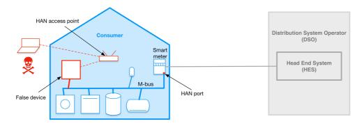
Figure 4.6: An attacker hacks into HAN and adds a virtual and malicious device to the M-Bus.
