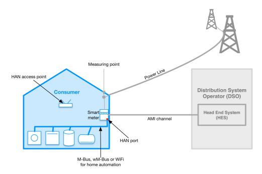
Figure 2.5: Illustration of the Smart Metering System.
