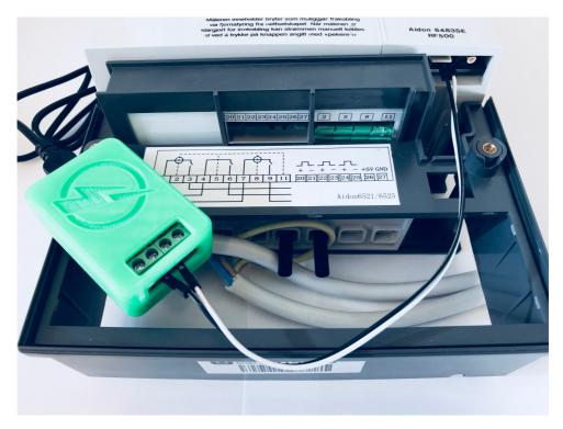
Figure 5.4: The green box is the M-Bus adapter that is connected to the HAN port. The white wire is used for ground, while the black wire is used for M-Bus. The other end of the adapter has a USB connector that goes to the computer.
