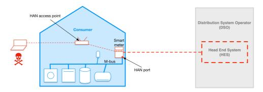
Figure 4.7: An attacker gains access to the smart meter via the HAN and is skilled enough to operate on a low layer, for example the data link layer, to get around the two-person check in order to turn on the breaker functionality.
