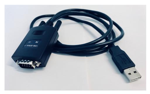
Figure 5.3: This picture shows the second RS232-to-USB adapter that was tried out in the primary test setup.
