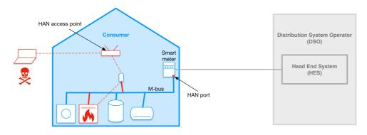
Figure 4.9: An attacker gains access to the third-party equipment via HAN and a controlling device. The attack could cause a fire if the electrical equipment is manipulated to be always on.
