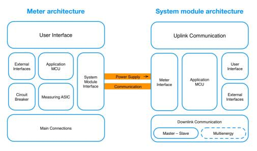
Figure 3.2: The architecture of the meter and the system module inside the smart meter. The figure is remade from an illustration received from Rolf Pedersen in Aidon [50].
