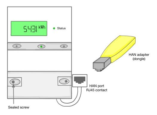
Figure 2.6: Illustration of the smart meter, the RJ45 physical contact and a HAN adapter to connect the home automation devices to smart meter. Inspired by [50].
