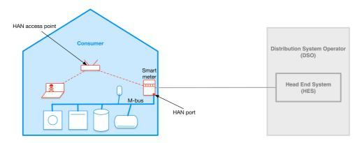
Figure 4.8: An attacker gains access to the smart meter via the HAN. The ping attack is aimed to overload the microcontroller unit (MCU) so that the smart metering system stops working.
