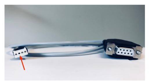
Figure 5.1: This picture shows a 4-pin connector where the missing pin is marked with the red arrow. The other end of the cable has a RS232 connector.
