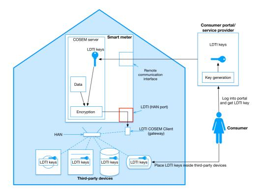
Figure 3.6: This illustration of the security environment using encryption has been inspired by [20, 51].
