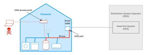
Figure 4.3: An attack via a third-party device by exploiting the operating systems in order to carry out an buffer overflow attack to make the system unavailable.
