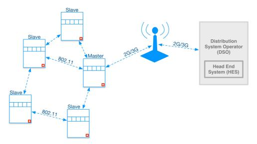
Figure 2.4: Illustration of the the mesh topology of smart meters. One of the meters is the master node that transmits and receives signals from slave nodes to the HES and the other way around. Inspired by [4].
