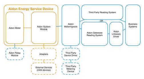
**Figure 3.1:** Overview of Aidon's Advanced Metering System which has been remodeled, inspired by [1, 4]. The thesis is concentrated around the Aidon Energy Service device (the smart meter) and the communication interface it has between adapters and external devices. This has been marked in orange.
