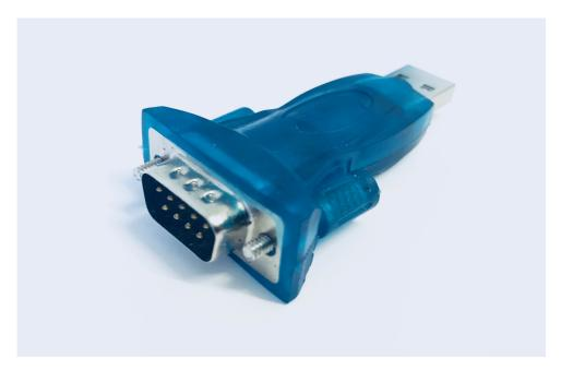
Figure 5.2: This picture shows the first RS232-to-USB adapter that was tried out in the primary test setup. This adapter was not possible to use.
