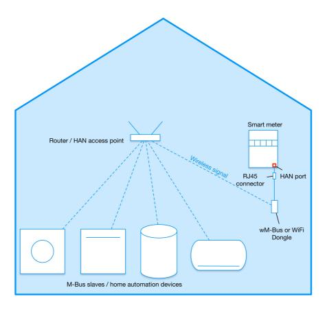
Figure 3.5: Getting data out of the HAN port with a M-Bus converter.
