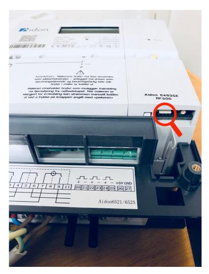
Figure 3.3: The smart meter borrowed from Aidon. The magnifying glass is circling the HAN port.
