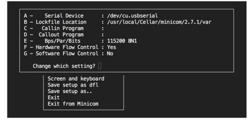
Figure A.1: Serial port setup in Minicom.
