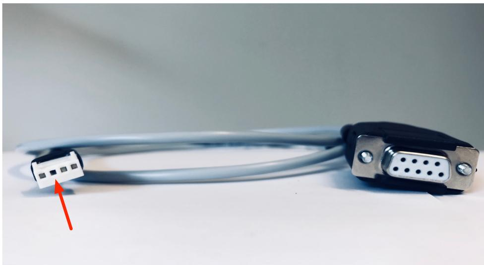
**Figure 5.1:** This picture shows a 4-pin connector where the missing pin is marked with the red arrow. The other end of the cable has a RS232 connector.
