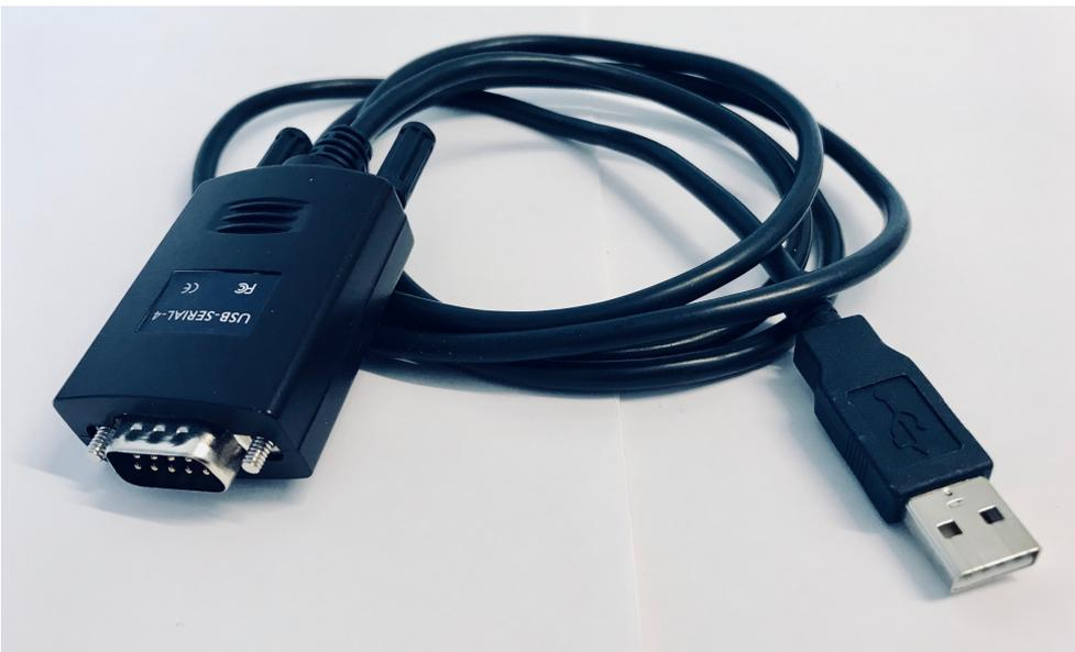
**Figure 5.3:** This picture shows the second RS232-to-USB adapter that was tried out in the primary test setup.
