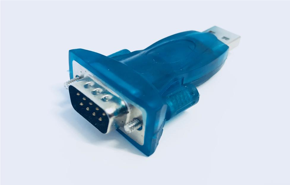
**Figure 5.2:** This picture shows the first RS232-to-USB adapter that was tried out in the primary test setup. This adapter was not possible to use.
