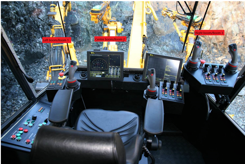
Figure 1.3: View from rig cabin. Drill booms marked with names. Courtesy of AMV
