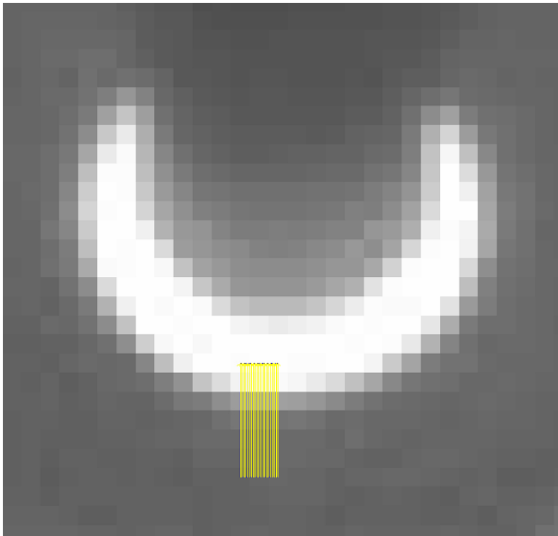
Figure 6.8: The LineFinder2 tool failing after being placed 1px further down on the image from Fig. 6.7b.
