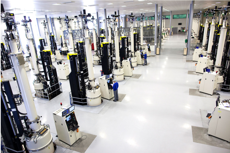
Figure 1.3: The NorSun factory's Czochralski pulling area. NorSun (2018)
