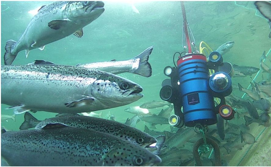
Figure 5.16: The SEALAB AquaPod with the Raytrix R42 camera attached. Photo: SEALAB.
