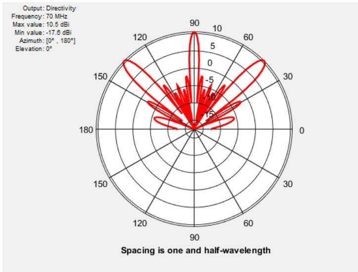
**Figure 3.2:** Visible grating lobes at 1.5 wavelength spacing [6]
