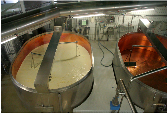
Figure 5.28: Open top curdling vats where the milk proteins are denatured into cheese. These are not the actual curdling vats we are reviewing in this task. Retrieved from Wikipedia 52 under the Creative Commons 3 licence 39 .
