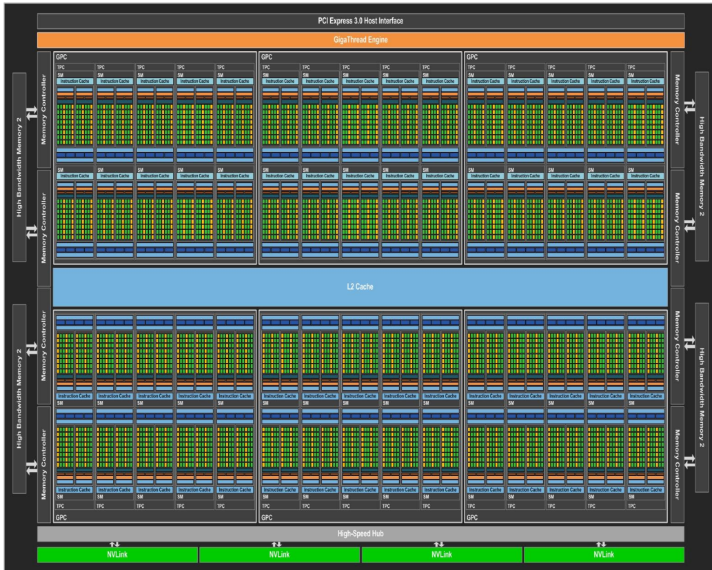
Figure 2.1: Overview of the Nvidia Pascal GP100 GPU with 60 SM units. From Nvidia Corporation [21, Figure 7]. Reprinted with permission.
