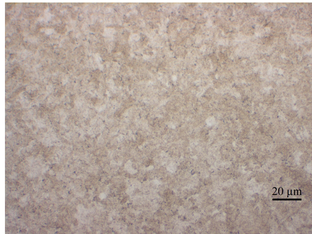
Figure 41: Micrograph of austempered 100Cr6 (3.B). Etched with Viellas etchant. Few prior austenite grains were visible. Magnification: 500x.
