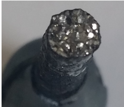
Figure 46: Fracture surface of austempered 100CrSiMn6-5-4 (4.B*). The sample was austenitized 30 min at 1200 °C, then 10 min at a lower austenitizing temperature before quenching.
