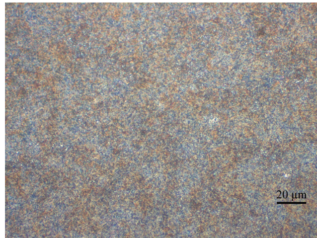
Figure 44: Micrograph of austempered 100CrSiMn6-5-4 (4.B). Etched with Viellas etchant. Few prior austenite grains were visible. Magnification: 500x.
