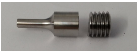
Figure 26: Cutting of tension rod. The part to the right was warm molded with cutting side down.
