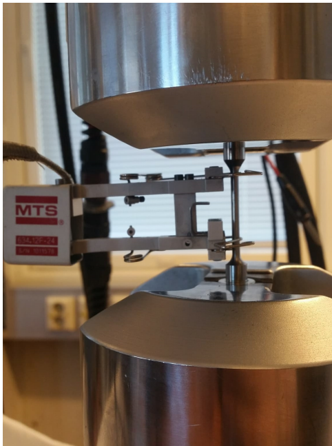
Figure 35: Tension rod in the testing machine with attached extensometer.
