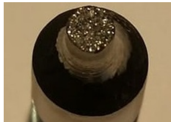
Figure 43: Fracture surface of austempered 100Cr6 (3.B*). The sample was austenitized 30 min at 1200 °C, then 10 min at a lower austenitizing temperature before quenching.
