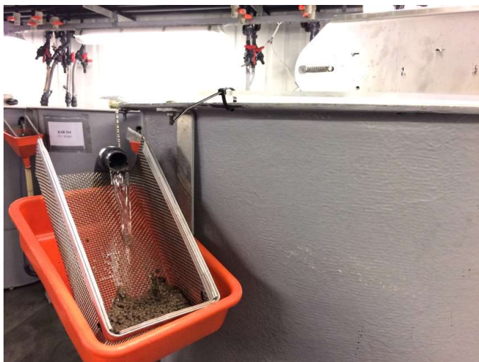
Figure 3.3 Sampling point, effluent water from a fish tank outlet.
