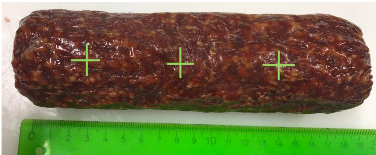
Figure 4.5-1: The crosses indicate where pH was measured approx. in the centre of the sausage. The length of the sausage is indicated on a sausage after drying.
