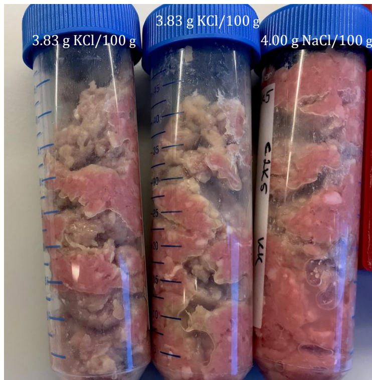
Figure 5.2-5: Tubes with meat mixture fermented with starter culture T-SPX for 5.3 days. The tubes containing KCl show the brown-grey patches that developed in these tubes.
