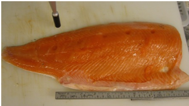
Figure 11: Texture analysis. The photo shows an Atlantic Salmon ( Salmo salar ) fillet being analysed with a Stable Micro Systems Texture Analysator, TA-XT plus.
