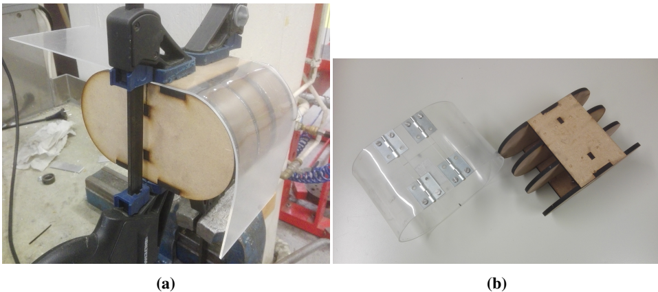
Figure 5.13: Production of PMMA prototype
