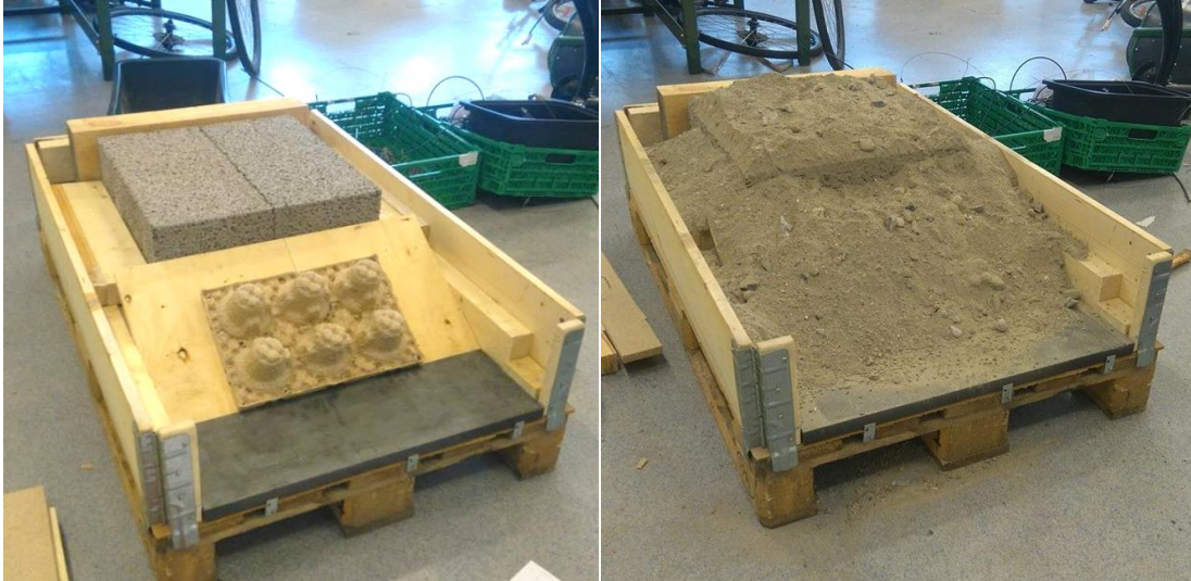
Figure 4.6 Pallet prototype featuring the most basic effects relevant to meet the objective.
