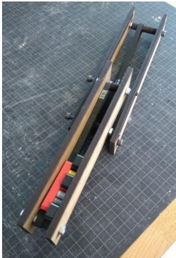
Figure 4.21 Rapid prototype of the telescopic links moving relative to one-another. Screws work as sliding bearings in a slot on each side of the lower bearing.
