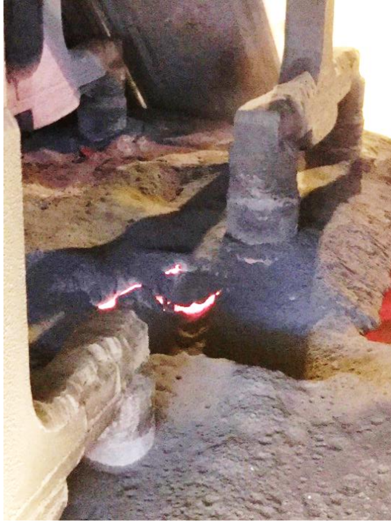
Figure 3.8 Example where cavities appear at the anodes' rear end.
