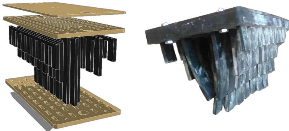
Figure 4.9 The rubber fingers tool was first made with rapid pattern features in CAD then cut accurately in a laser cutter.
