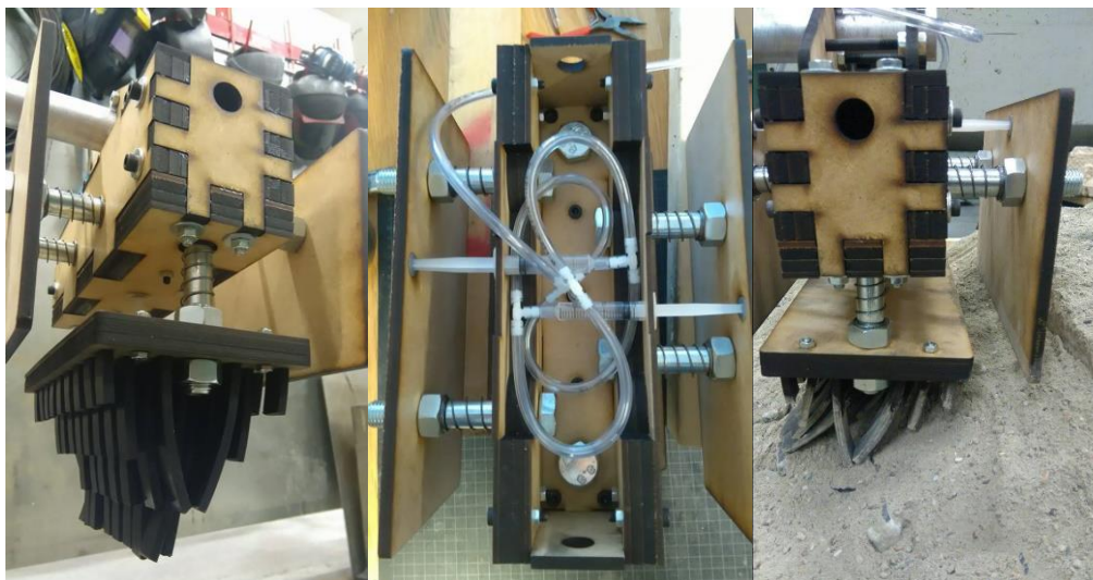
Figure 4.28 The handheld rubber fingers tool. The previously visited tool attached to a center-box (tool-center) for bolt-wandering when the pre-compressed springs gets further compressed (left). A common pneumatic system for two crash-impact plates, front and back, and the vertical impact from the surface interaction (middle). The tool was applied in the pallet prototype (right).
