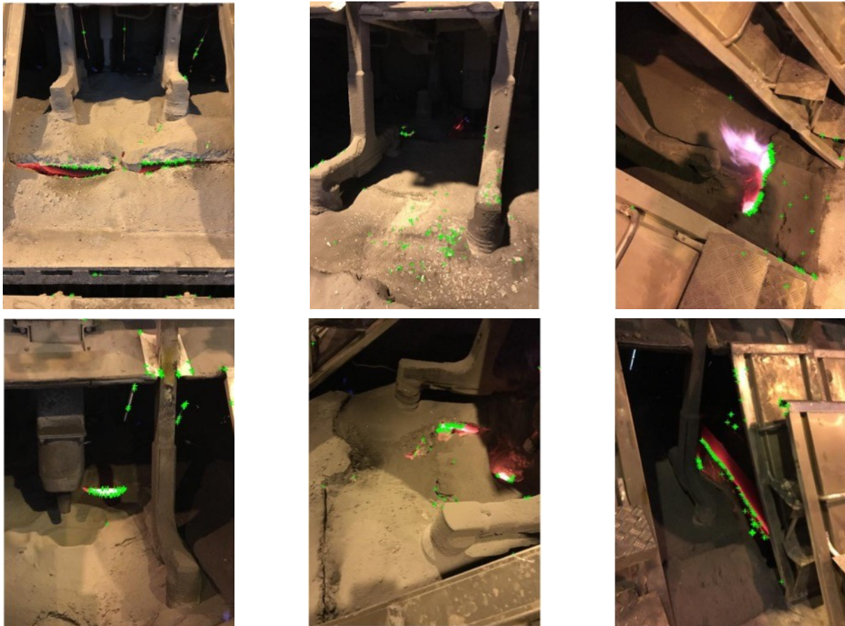
Figure 12: Applied Harris corner detection algorithm on pot images in MATLAB.
