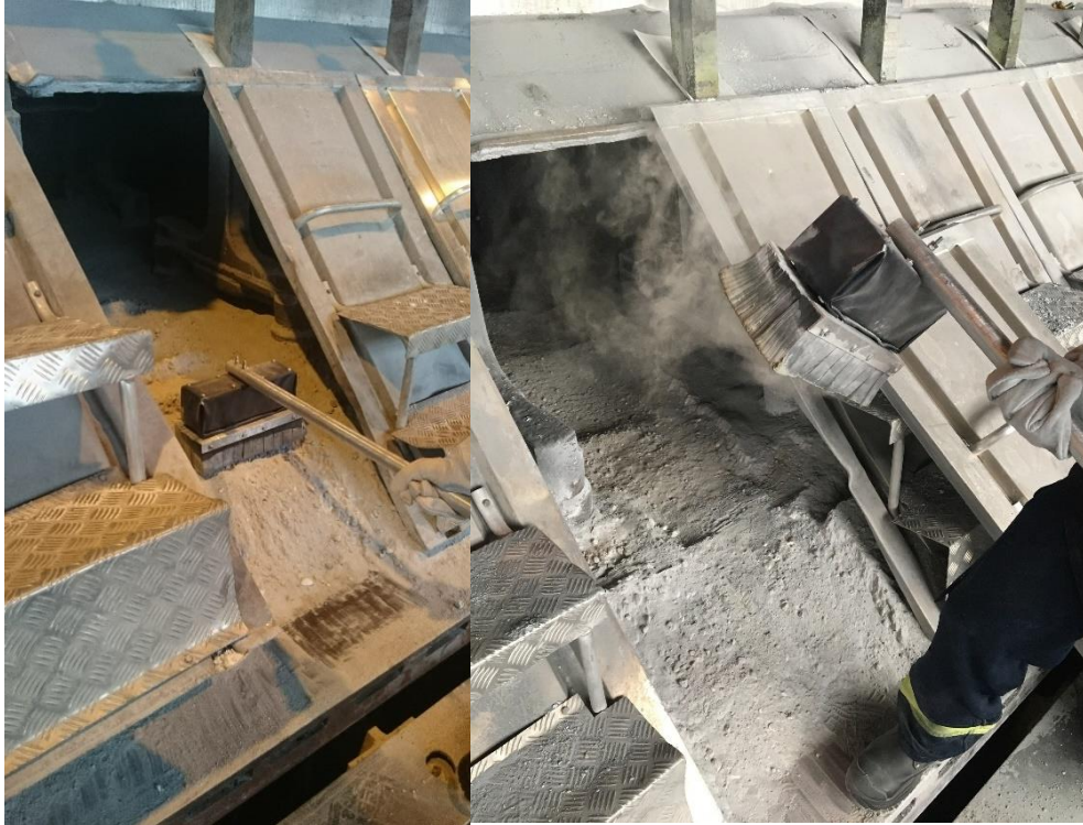
Figure 4.33 The rubber fingers tool applied for anode covering during pot tests at the corporate partner. Dust and rubber-smoke is clearly seen in the picture to the right. The tool did however perform well with respect to its mechanical principle but still lacking a certain stiffness.
