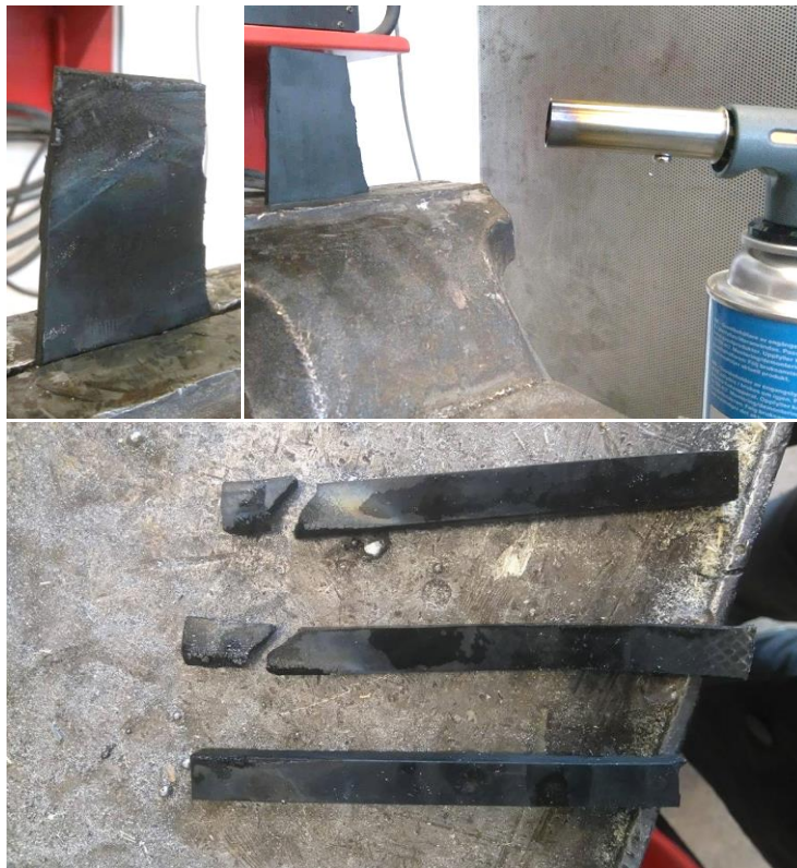
Figure 4.16 Torch-testing rubber strips with respect to the rubber-fingers-tool test. The degradation is first prominent with applied load. Setup (top, right), burnt, wide specimen (top, left) and burnt and fracture strained slim specimens (bottom).
