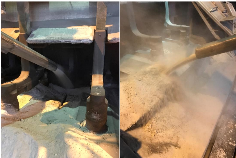
Figure 3.3: Feeding of cover-mass on newly inserted anodes.
