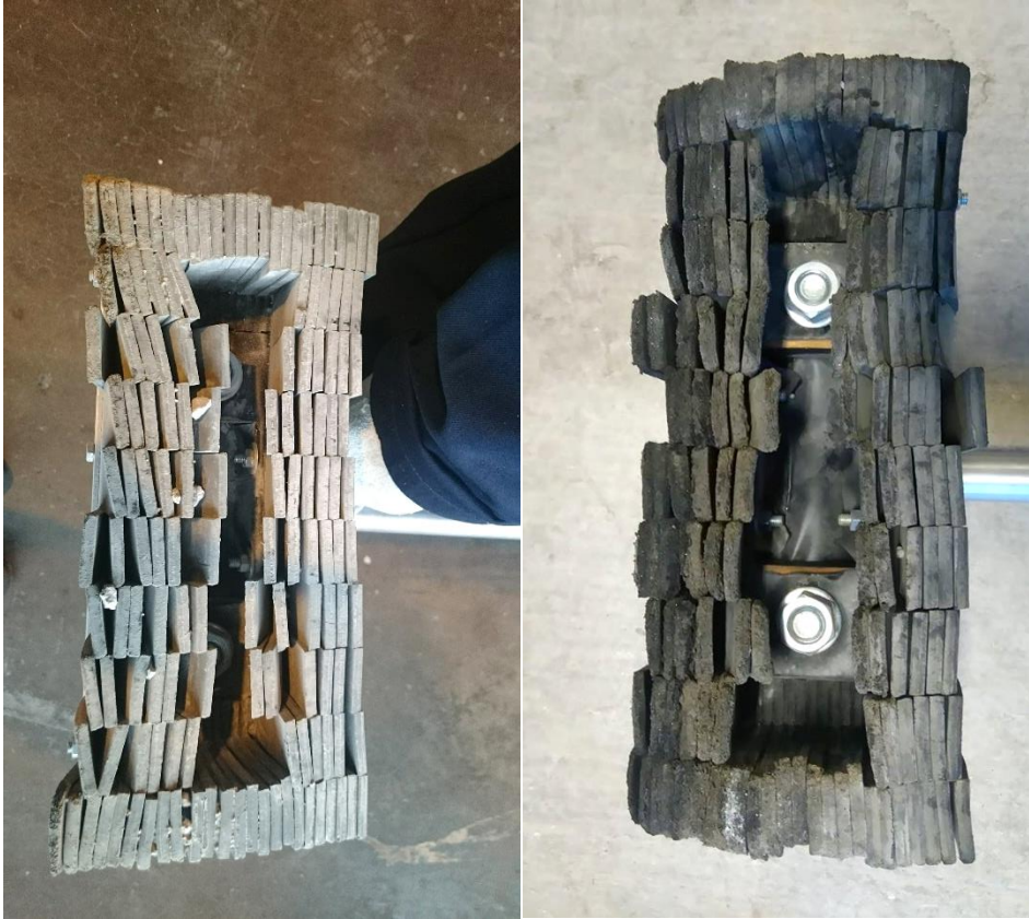
Figure 4.34 The rubber fingers tool seen from below. Only one iteration showed some degrading in the fingers and fine gravel getting stuck (left). After several runs of covering and intentional, destructive testing in open pot fires, the rubber fingers were shattered (right). A marked difference between front and back gives an indicator on the mechanical shear's impact when heated, as most load was applied in the front.
