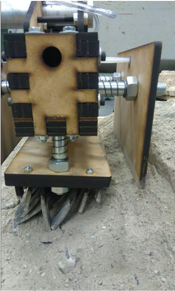
Fig. 6. Product prototype for ultimately performing anode covering autonomously. Several solutions for different functions are here combined.
