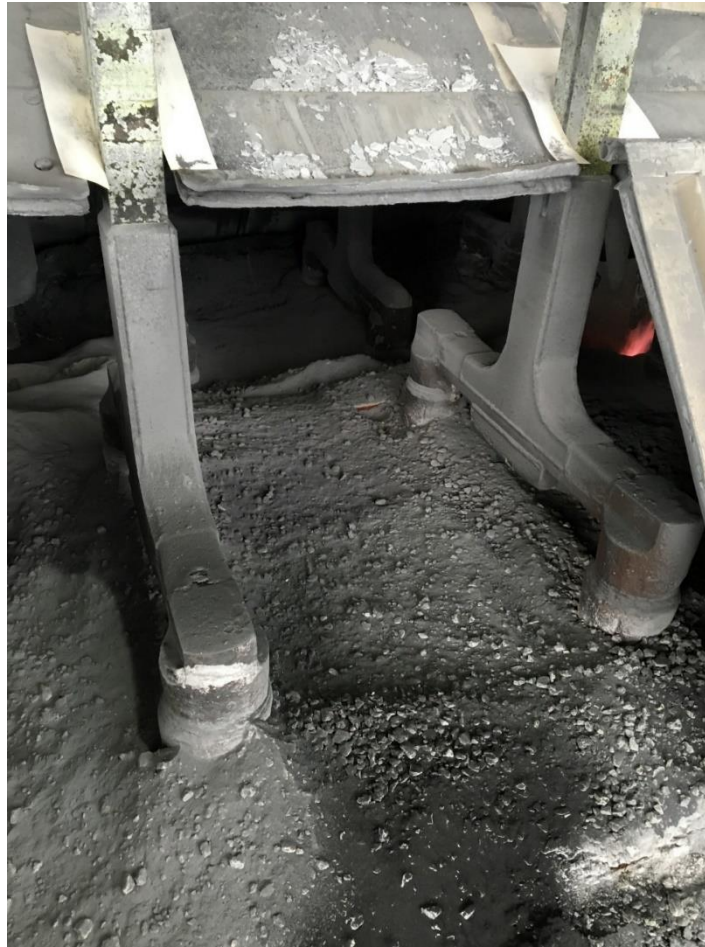
Figure 3.7 Decent surface conditions and a common scene in the first half of the anodes' life-cycle.
