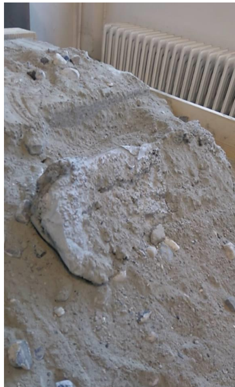
Figure 4.10 The casted concrete "crust" partly covered within the pallet prototype.
