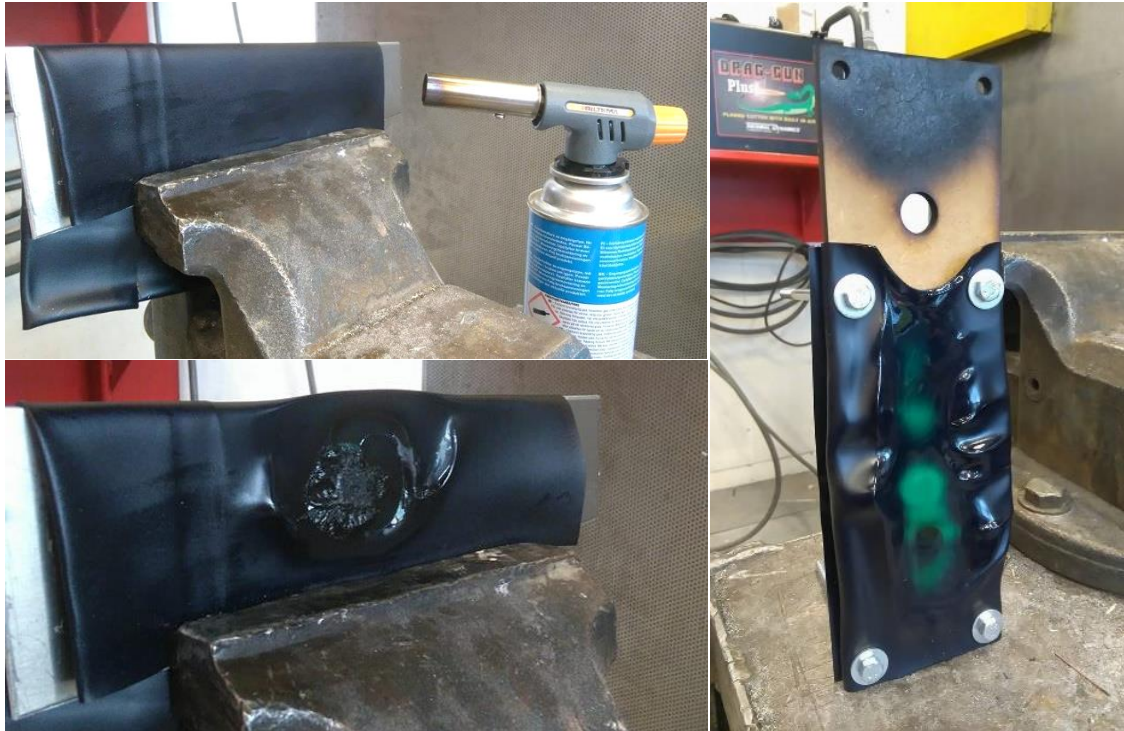
Figure 4.17 Torch-testing MDF with and without a flame-inhibiting welding curtain for cover. The curtain degrades fast during torching due to its excellent absorption of energy. Setup (top, left), Curtain-test (bottom, left), MDF-test (right).
