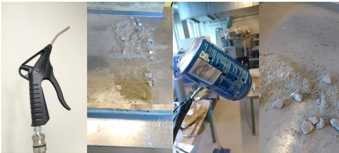
Figure 4.3 Air pressure pistol applied for moving cover-mass on metallic surface. Conditions after testing are shown. A diffuser can was applied in the iteration to the right.
