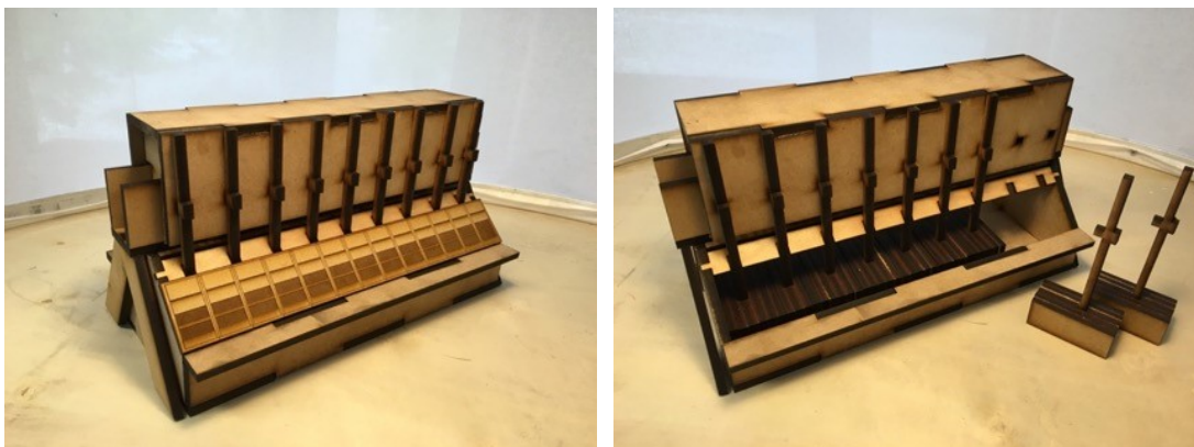
Figure 6: Demonstrator prototype of aluminium melting pot made out of laser cut MDF
