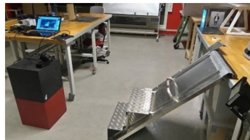
Figure 14: Cover-image-processing test setup. A Microsoft Kinect V2 and a Grundig mini-projector are placed 1.5 meters from the cover handle, with the Kinect camera at about the same height.
