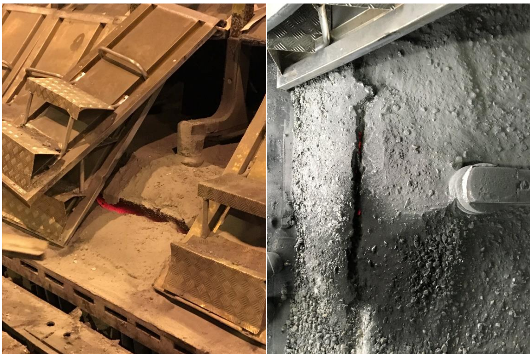
Figure 3.6: The scenario of cover-mass on the front plate and exposure or cavities in front of the anode.
