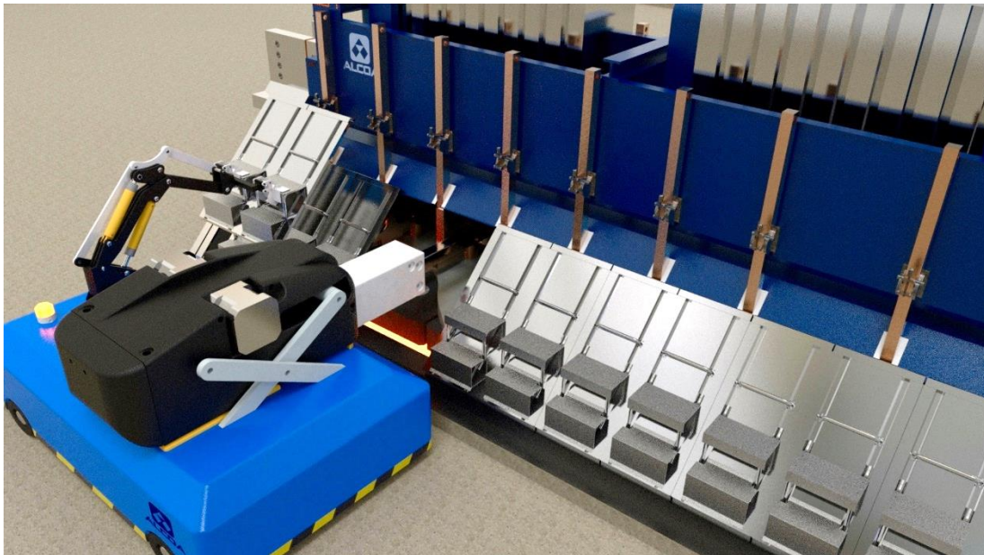
Figure 5.1 The Cartesian concept together with Even Jørs' concept-unit for cover-handling operations together on an AGV.
