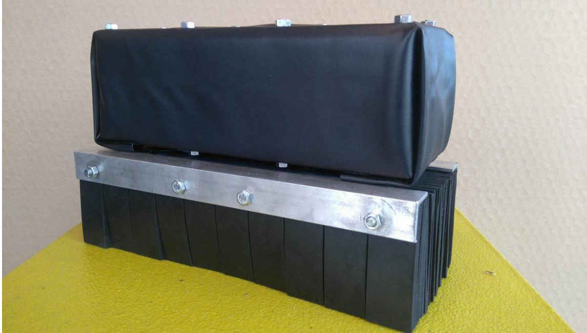
Figure 4.31 The rubber fingers tool. Featuring a tight grid of clamped rubber fingers. The clamping gives simpler design for assembly. The fingers are wider and shorter from last iteration for higher stiffness, and in terms with the findings from the torch test. A box in MDF is covered within the wrapped welding curtain.
