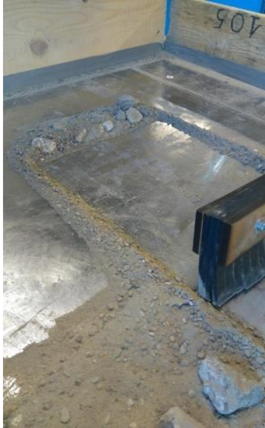
Figure 4.4 Clamped natural rubber was used to sweep the metallic surface with excellent results.
