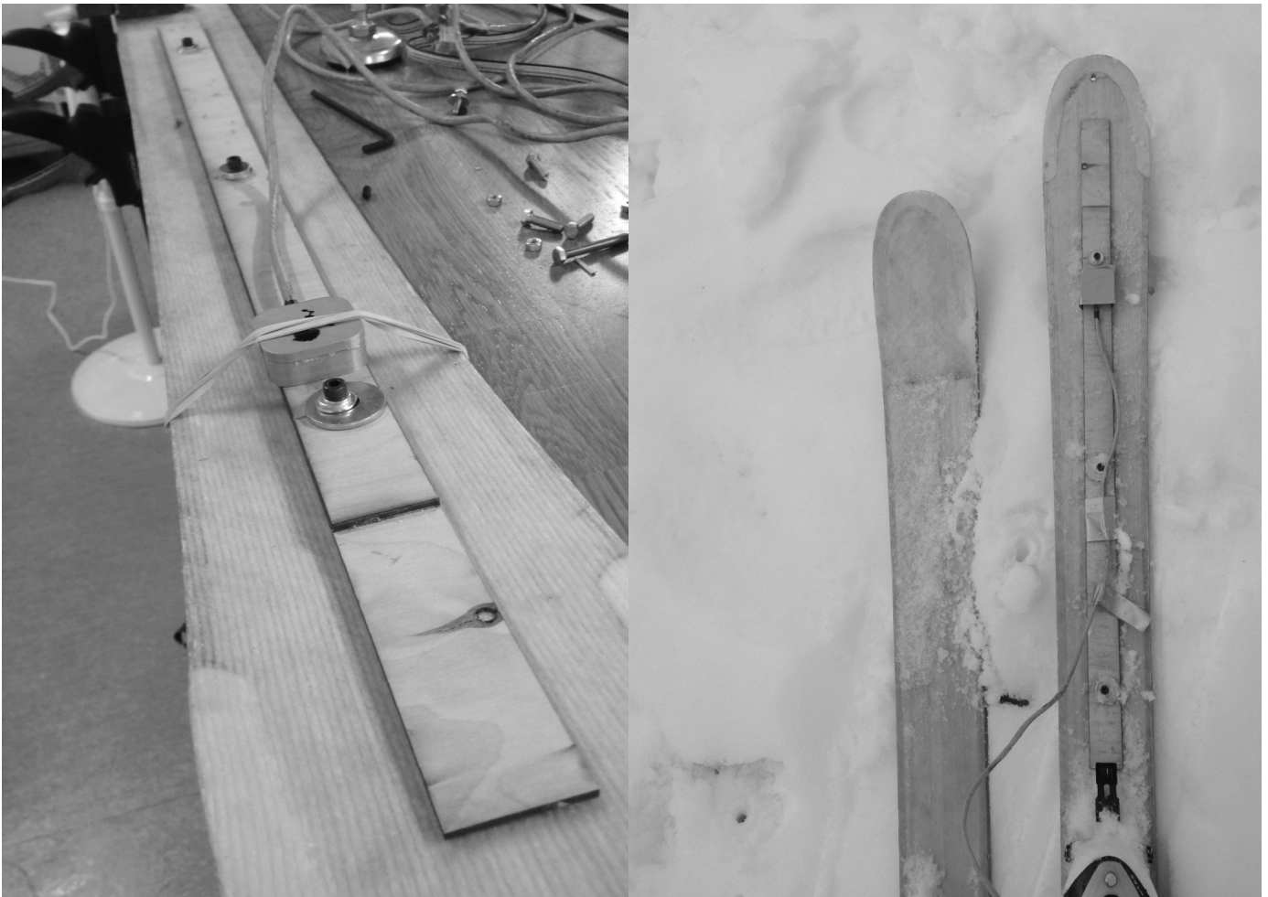
Figure 21: (A): Prototype of adding stiffness by increasing moment of inertia. (B): Testing the setup in (A).
