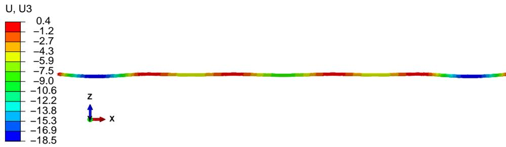
Figure C.51: Z-deformation. Tugboats with 35 tonnes towing force. Deformed shape
