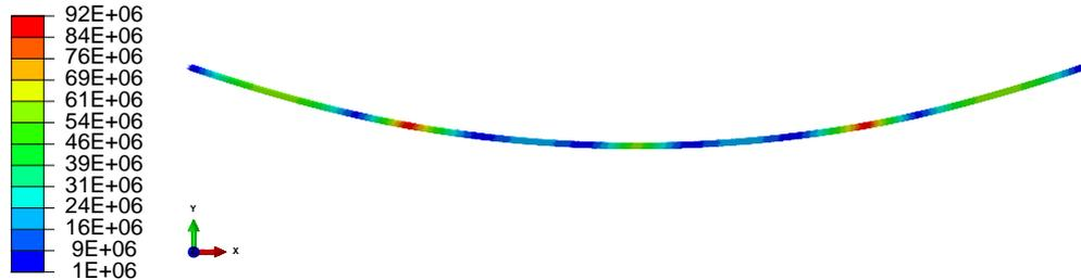
Figure 5.5: 3 barges, von Mises stress in bundle
