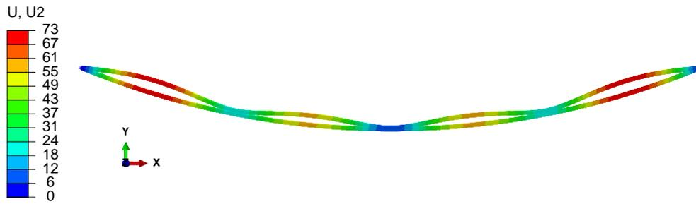
Figure C.36: Y-deformation. Tugboats with 50 tonnes towing force. Deformed and initial shape
