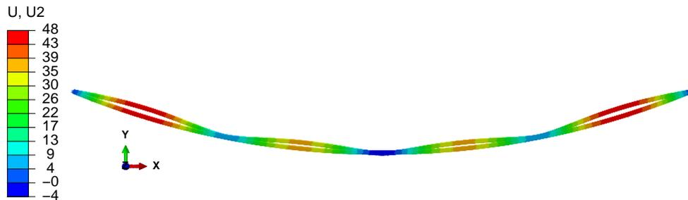
Figure C.47: Y-deformation. Tugboats with 60 tonnes towing force. Deformed and initial shape
