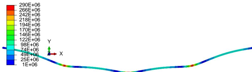
Figure 5.4: Von Mises stress for bundle with 3 tugboats with 55 t force
