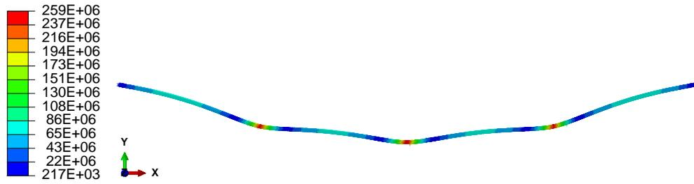
Figure C.46: von Mises stress. Tugboats with 60 tonnes towing force
