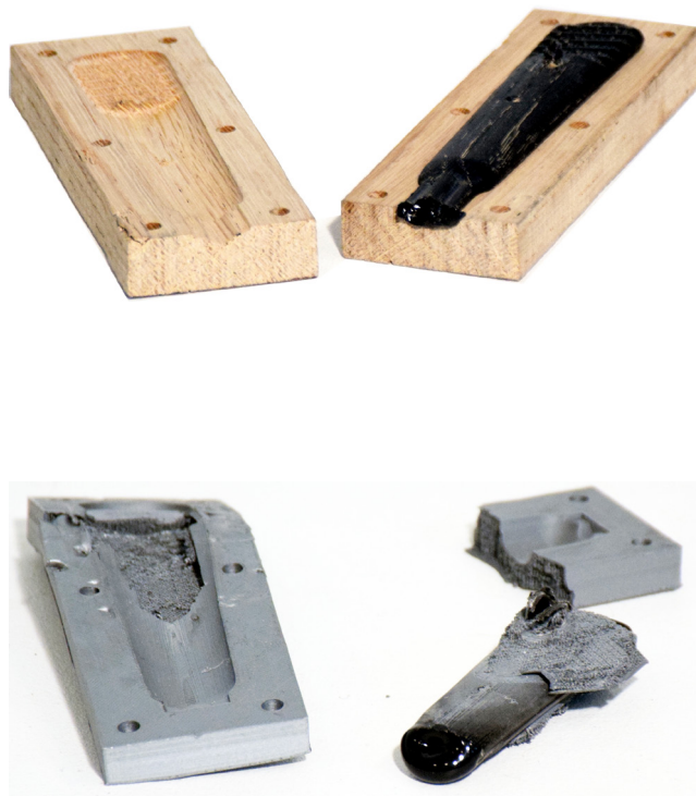
Figure 32: The results from the Wood mold (top) and Aluminum Filled PLA mold (bottom).
