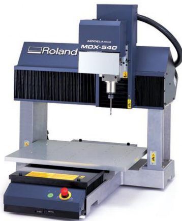
Figure 25: The Roland MDX-540 CNC mill. Photo courtesy of Roland.
