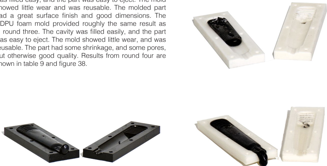
Figure 38: The VeroBlackPlus mold (left) provided good results. The Monochrome White mold (top right) melted upon injection. The Alloy 910 mold (bottom right) also provided satisfactory results.
