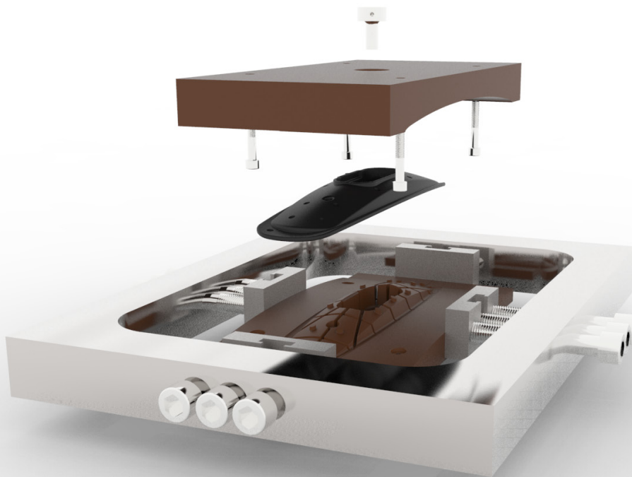
Figure 64: The tool insert method allowed for production level parameter control.
