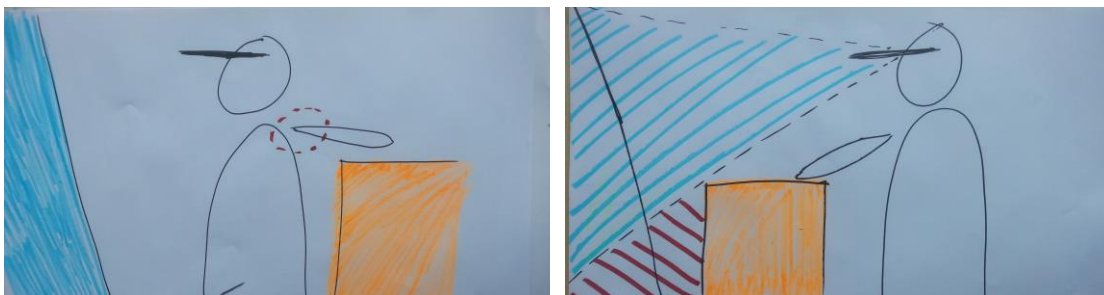
Figure 16: Left: Devices placed behind the user. Right: Part of view is hidden by console. The red hatched area is a blind zone.
