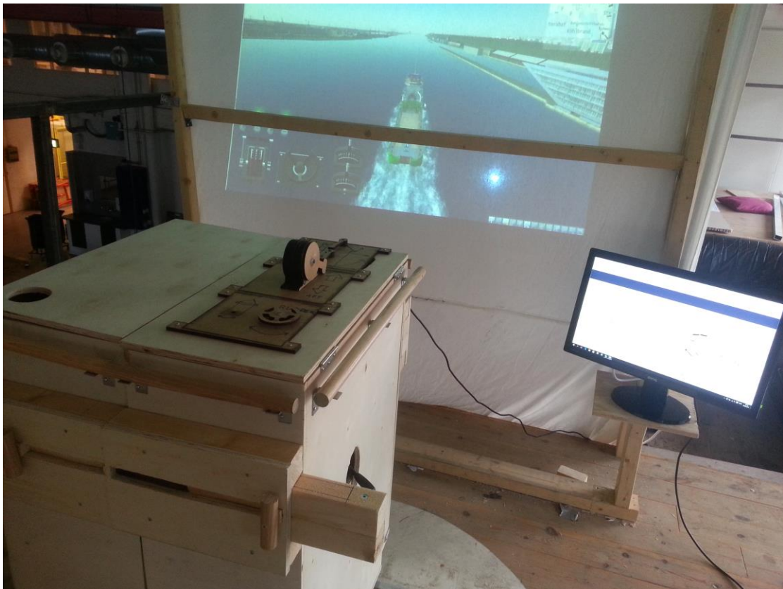
Figure 36: Setup for Experiment, Part II: Added body support and platform for ECDIS
