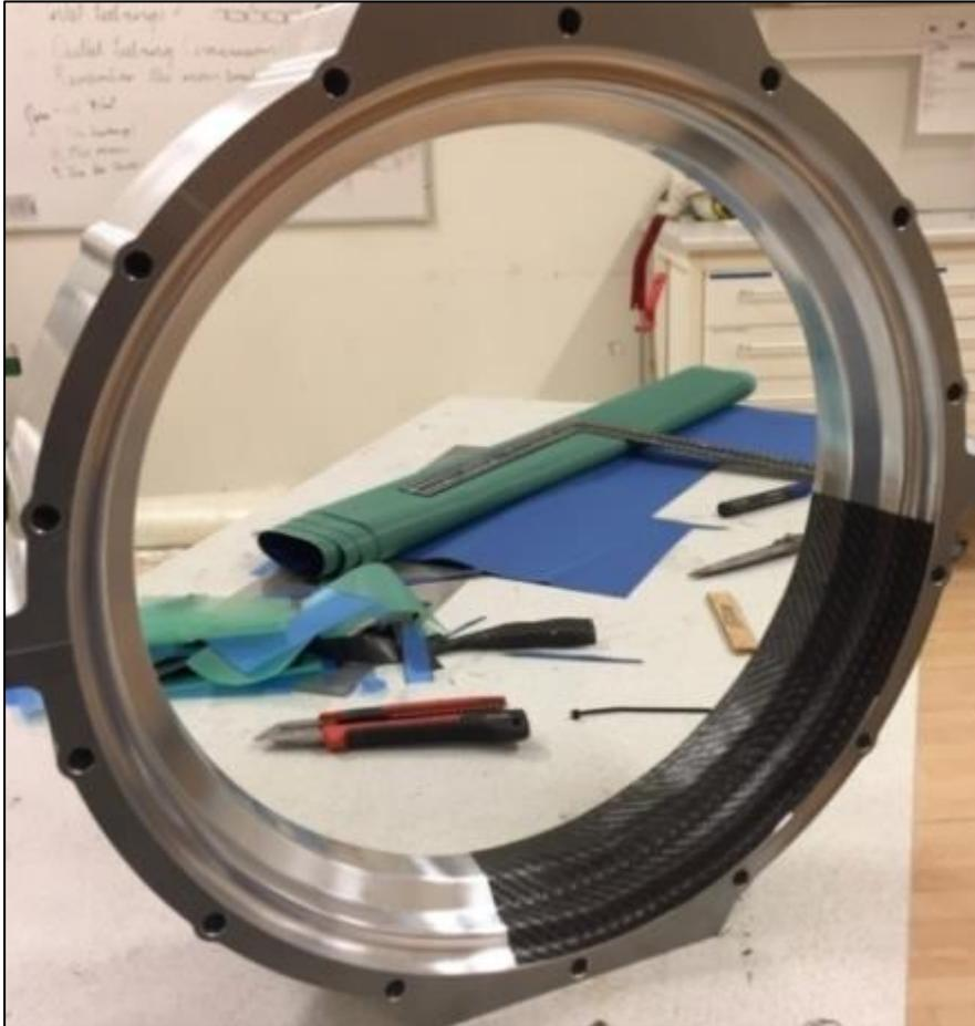
*Figure 4.13 The mould during layup of carbon fiber*
