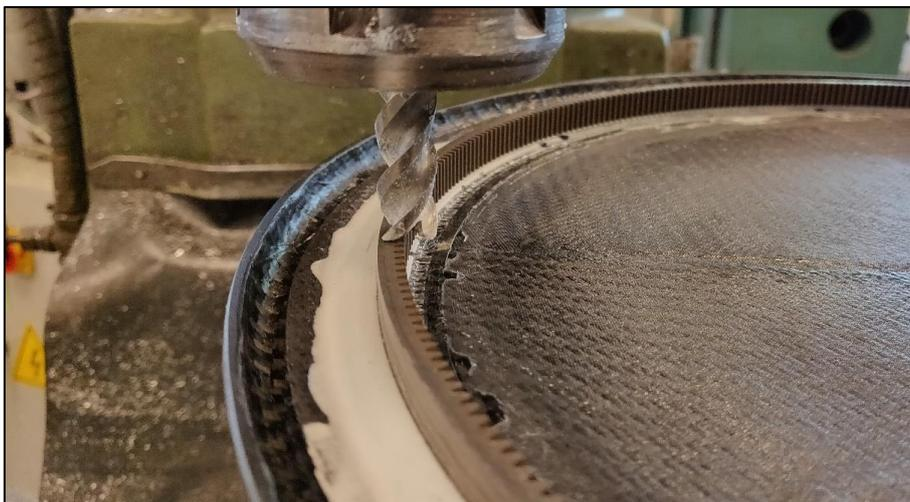
*Figure 5.29 Track cut out for gear with tight tolerance*
