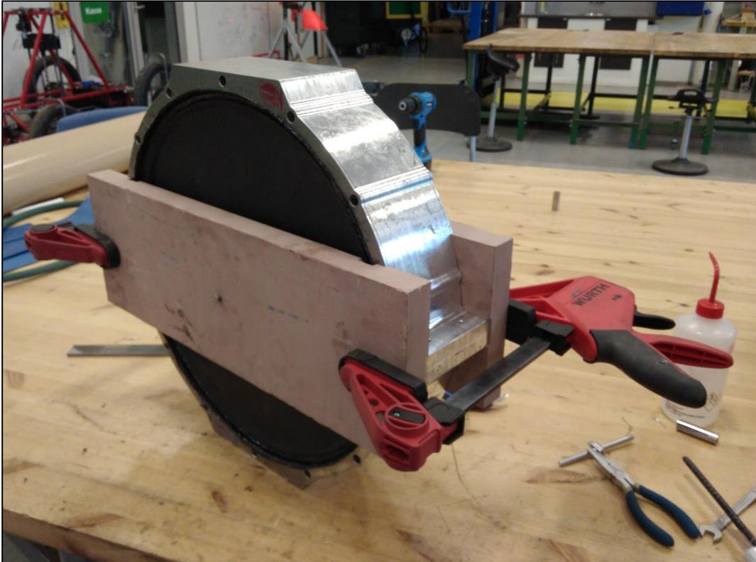
Figure 4.18 The centering tool fastened to the mould
