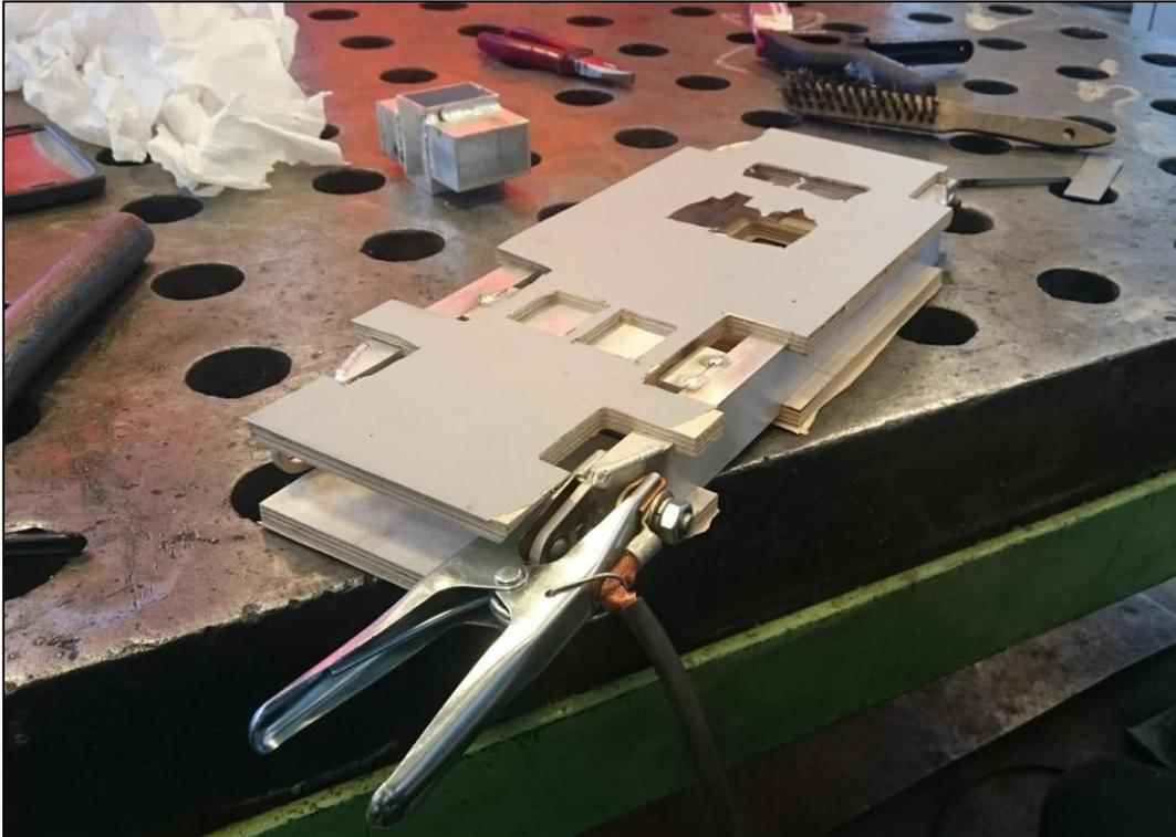
*Figure 5.24 Welding jig for the frame*
