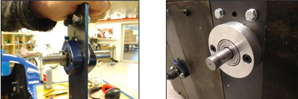
FIGURE 5-E OLD VS NEW BEARING HOUSING
