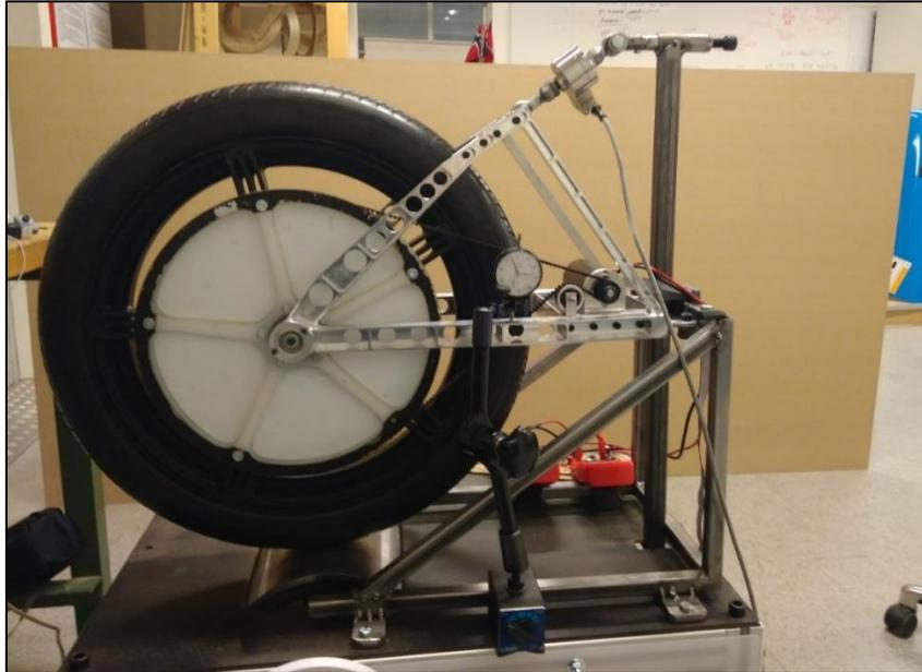
**FIGURE 5-A USING DIAL INDICATOR TO MEASURE DISPLACEMENT**
