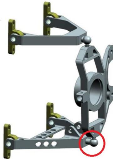
*Figure 8.3 The fractured part in the suspension system*
