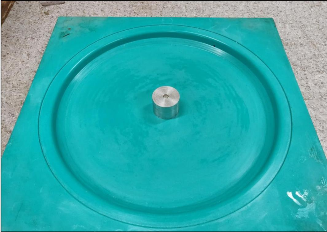
Figure 4.14 The finished center plate mould
