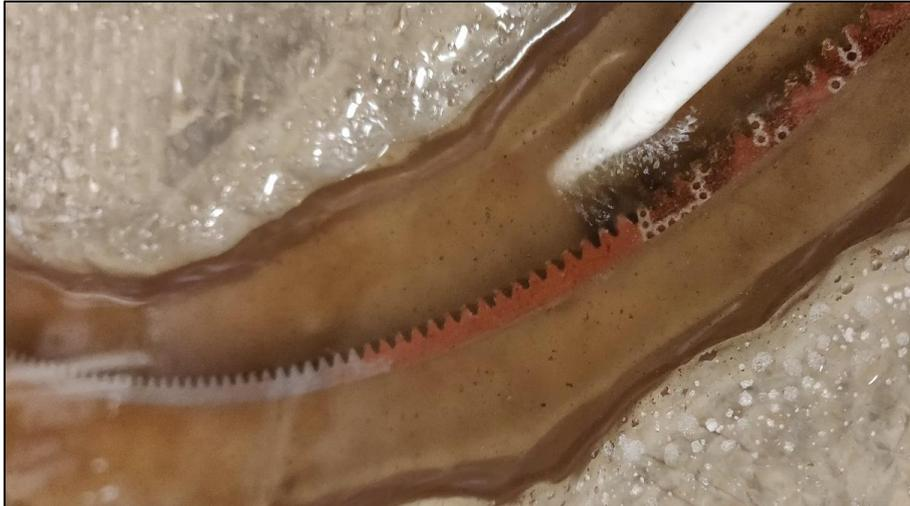
*Figure 5.27 Removing rust from the gears with vinegar, salt and electric toothbrush*
