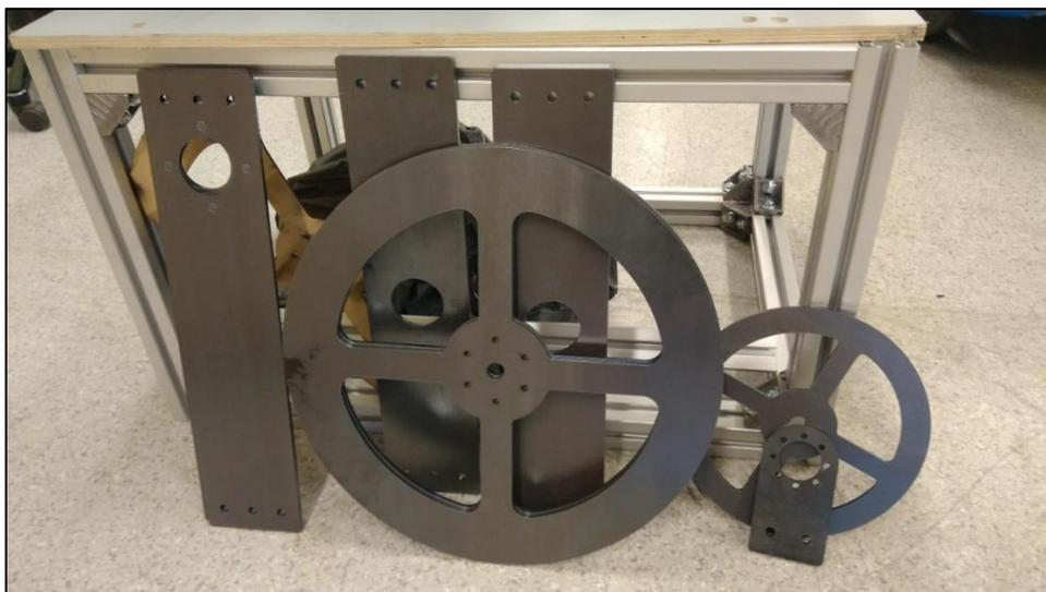
FIGURE 4-D THE PLATES READY FOR ASSEMBLY WITH THE MAIN FRAME IN THE BACKGROUND
