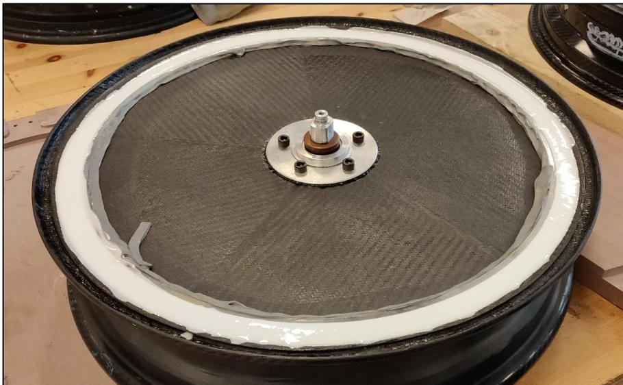
*Figure 5.28 Epoxy mixed with micro balloons added the rim with a lasercutted disc to hold micro balloons in place*
