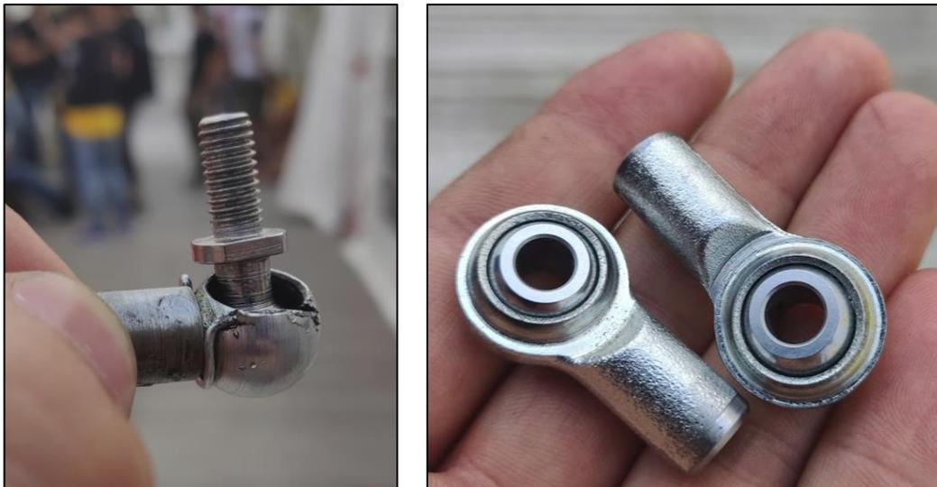
Figure 8.2 Fractured old ball joint vs. new Heim joints
