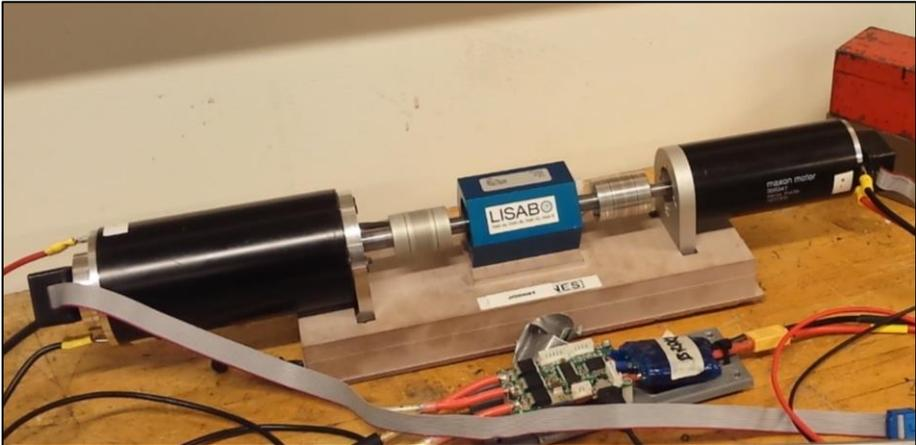
Figure 3.11 Two Maxon motors mounted in our test configuration
