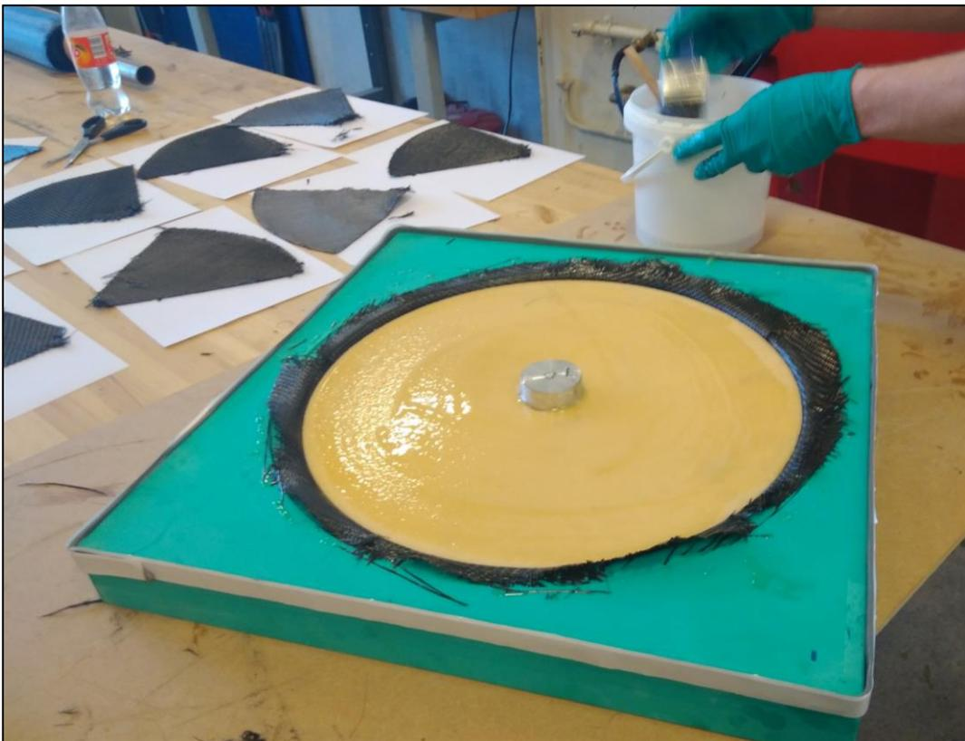
Figure 4.15 Lower layer and foam laid in the mould.
