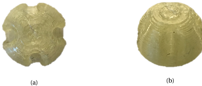
Figure 6.14: 3D-printed bladder core (PVA), with cavities creating laterally stiffening braces to the finished silicone mould.
