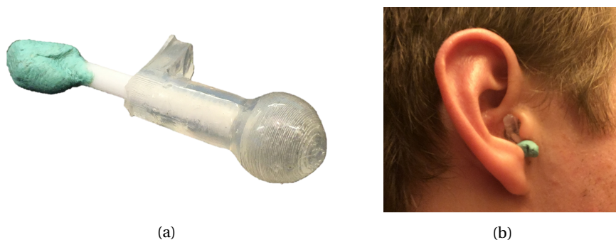
Figure 6.11: Testing the 1 st prototype of the bladder and stem in the EAC.
