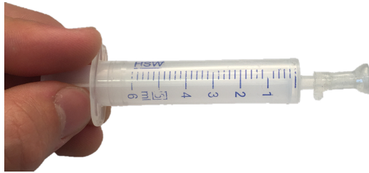
Figure 6.10: 1 st prototype with simulation of bladder contraction when evacuated.
