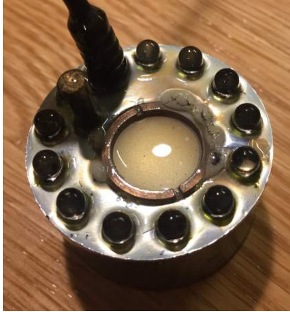
Figure 14: Accumulation of residue from the nutrient forming on the fogger
