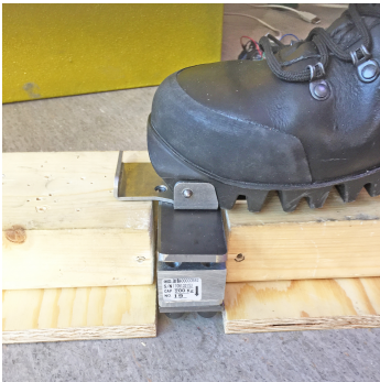
Figure 4-20: Measuring the forces straight up and down.
