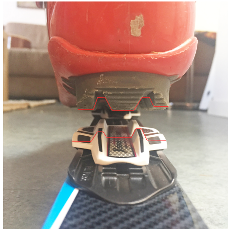
Figure B-14: A heel piece for a cross country ski binding. When a person is standing on the skis, the shoe will 'lock' into the heel piece since the shape of the shoe fits in the heel piece, this will support against any twisting motion of the shoe.
