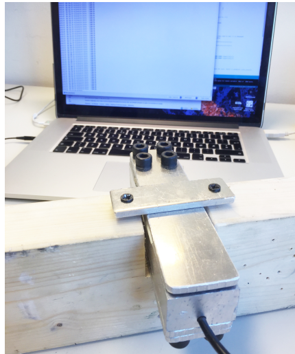
Figure 4-22: Measuring the force generated by pre-tension.
