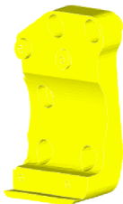
Fig. 20. Compressor bracket model for topology optimization
