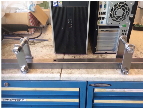
Figure C-24: For fastening the aluminium profile. Two rollers were constructed to make sure that only a vertical force was transferred through the binding.
