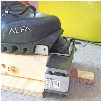
Figure 4-18: Measuring the force when the flex is compressed.
