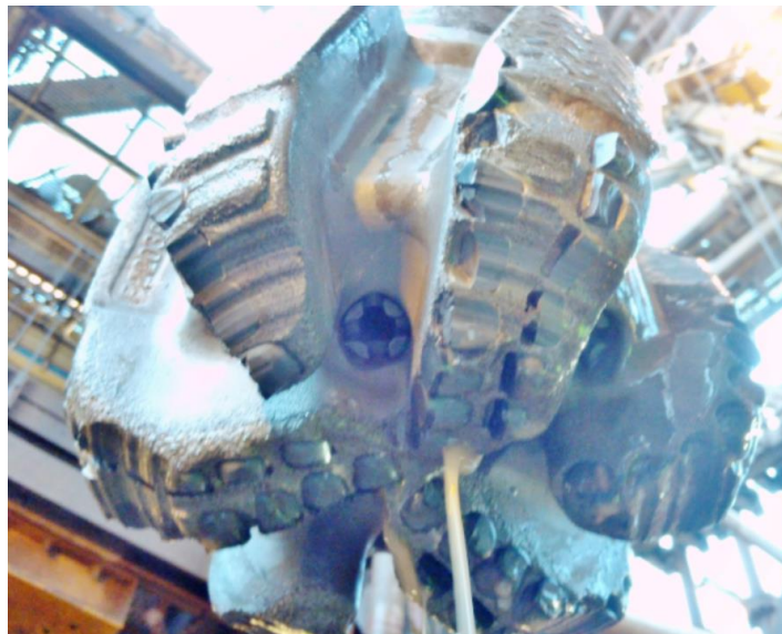
Figure 7.3: Worn cutters on the bit from Well B
