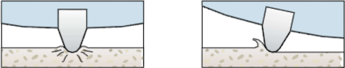
Figure 3.8: The mechanism of crushing (left) and scraping (right) (Brechan, 2015)
