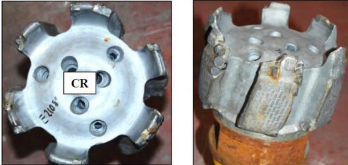
Figure 7.2: Completely worn bit from Well A
