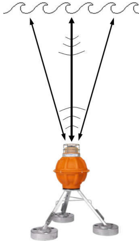
Figure B.1: Illustration of the principle behind the PIES. The PIES is deployed on the sea floor and emits acoustic waves. It measures the pressure and two-way traveltime, and calculates from this the water depth and the vertical average water velocity. The figure is acquired from Wang et al. (2012) .
