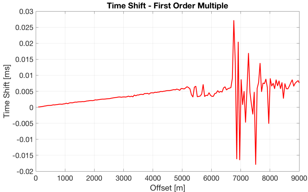
Figure 6.3: Raw time shift curve for the 1 st order multiple from the same shot gather as in Figure 3.4. Note the large spikes for 6500 - 7800 meters offset. This might be caused by seismic interference, which occurs in the same offset interval, highlighted by the red ellipse in Figure 3.4.
