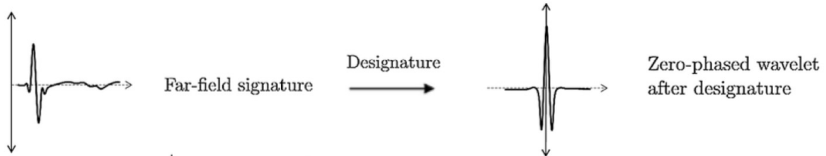
Figure 3.5: Conceptual illustration of designature. After a designature, the wavelet is shaped from the far-field signature to a zero-phase wavelet.
