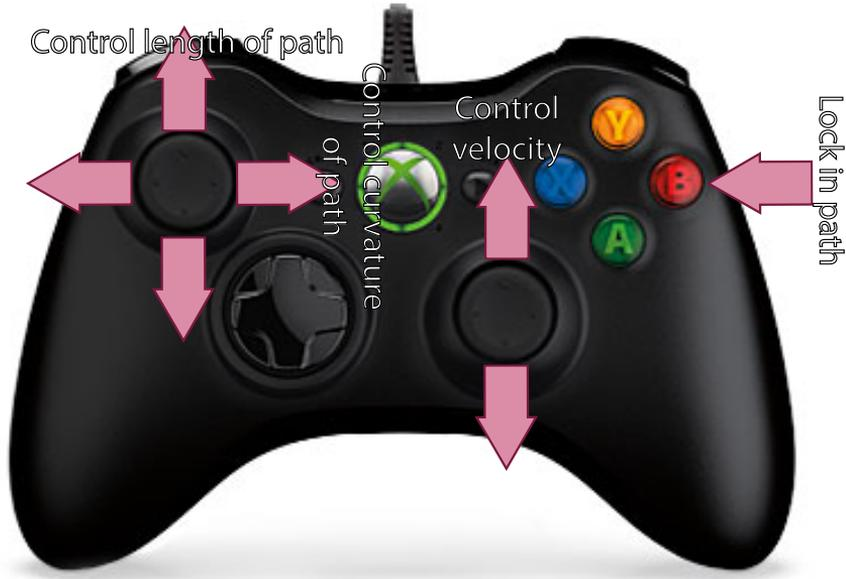
Figure 3.1: User input for path-following
