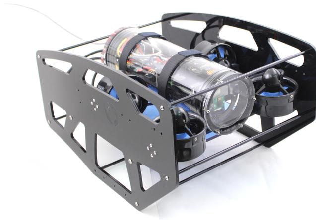
Figure 2.6: Blue Robotics BlueROV (source: bluerobotics.com)
