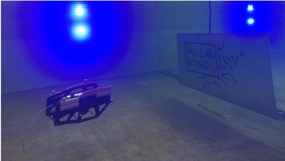
Figure 4.1: ROV uDrone in the Marine Cybernetics Laboratory basin during full DP using ORB-SLAM as position reference.
