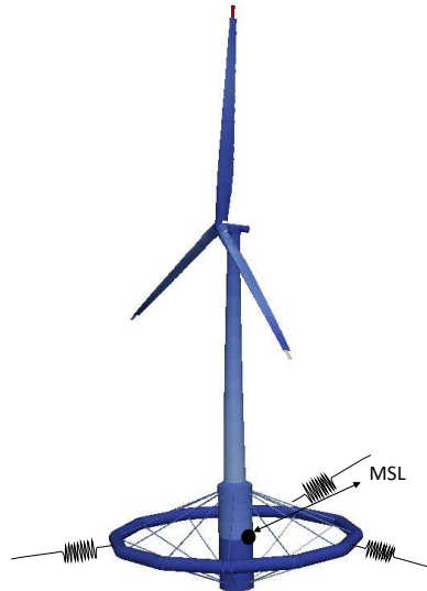
Figure 4.3: Mooring line formulation of the numerical model
