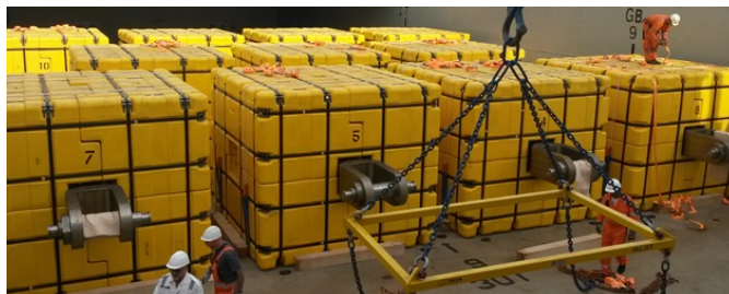
Figure 11.8: Mooring buoyancy elements (Lankhorst Mouldings)
