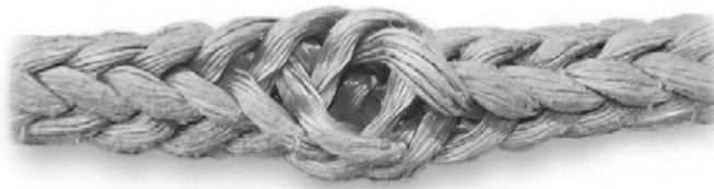
Figure 11.2: Fibre rope subjected to large compression forces (Smith 2011)
