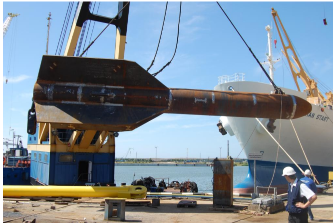
Figure 2.9: Deep penetrating anchor of 75 t (Deep Sea Anchors)
