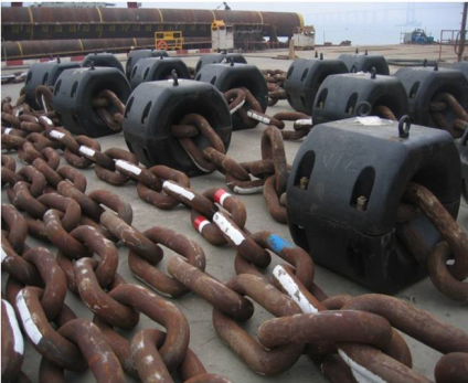
Figure 2.4: Clumpweights attached to chain (AMC)
