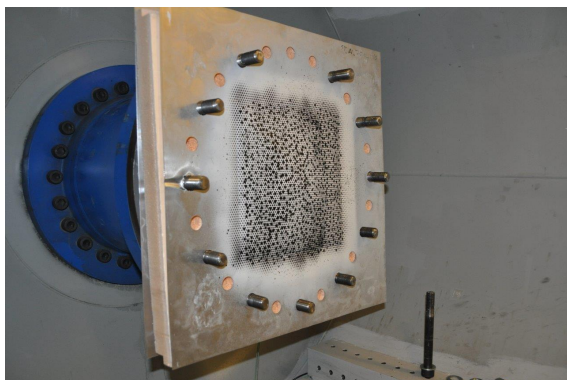
Figure B.9: Picture of front skin (top), foam (middle) and back skin (bottom left) deformation and the clamped component (bottom right) of sandwich panel with aluminum skins and XPS-700 foam core exposed to 10 bar firing pressure.
