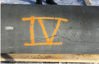
(a) Reinforced BASAL Falsrør ig subjected to 300 g C 4 . Exterior cracks visible in longitudinal and circumferential direction.
