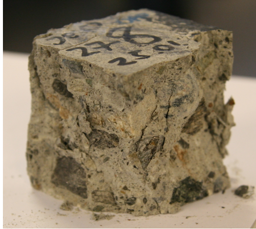
Figure 4.2 – Concrete cube used in experiments. Aggregates embedded in the HCP matrix are visible, and fracture is seen to occur on the surfaces of the aggregates, in the transition zone.
