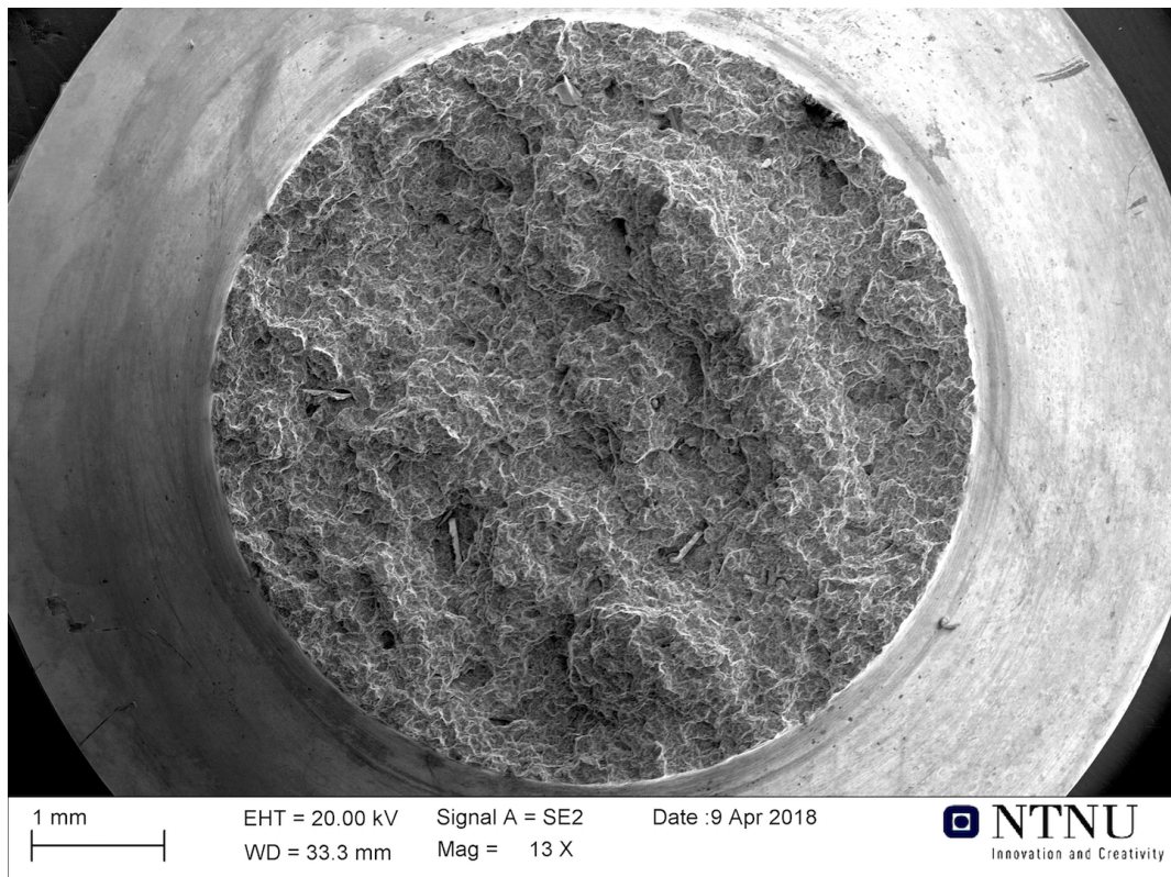
Figure A.10: Overview of the fracture surface for the V-notch specimen.
