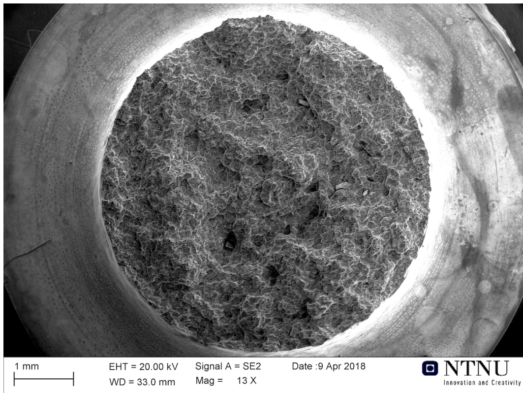
Figure A.7: Overview of the fracture surface for the R08 notched specimen.
