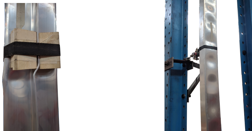
(a) Local buckling of the flange exposed to compression.
