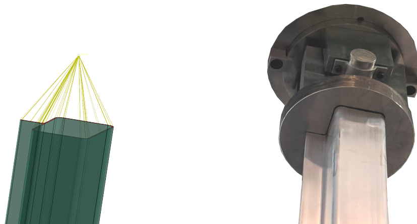
(a) Top support modeled in Abaqus. (b) Experimental setup of top support.
