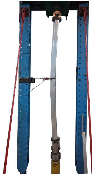
(b) Wire connected to column through pulley system.
