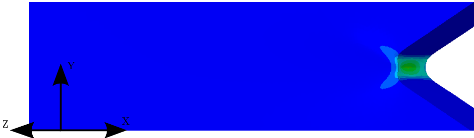
(b) Deformation at point 2a from Figure 4.35 with equivalent plastic strain. The test simulated is AA6082.25 WQ. The strain values are shown in Figure 4.34c.
