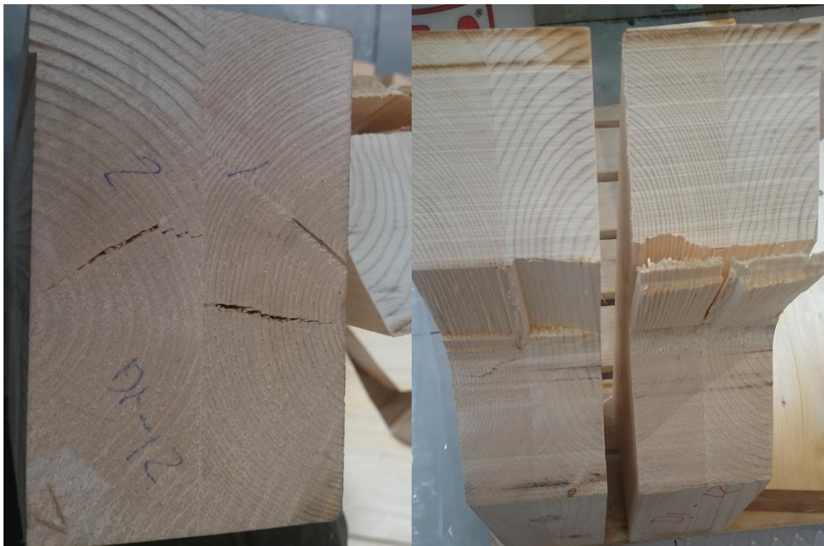
Figure 44-failure mode 2 due to drying cracks in shear plane causing deviation of fracture-plane.
