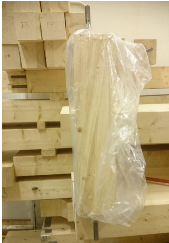
Figure 18 – Plastic bags used as vapor barriers, clamping in top and bottom
