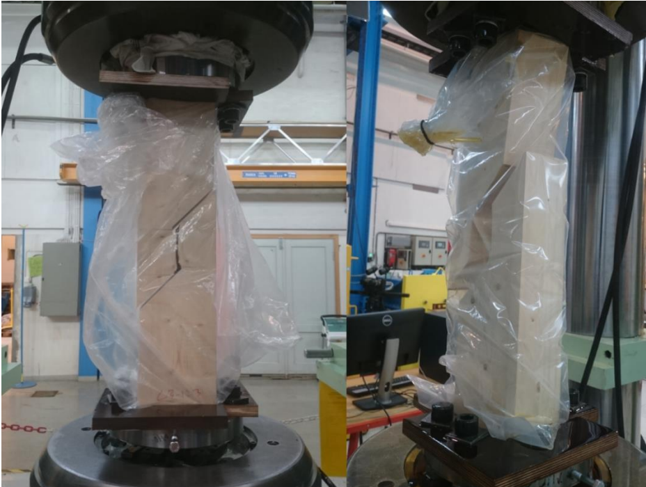
Figure 41-Vapor barrier used during testing
