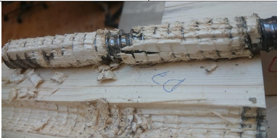
Figure 29-F0-D7-678, failure mode 3, follows intersection zone but deviates and tears out some fibers, it might seem to follow the annular rings..
