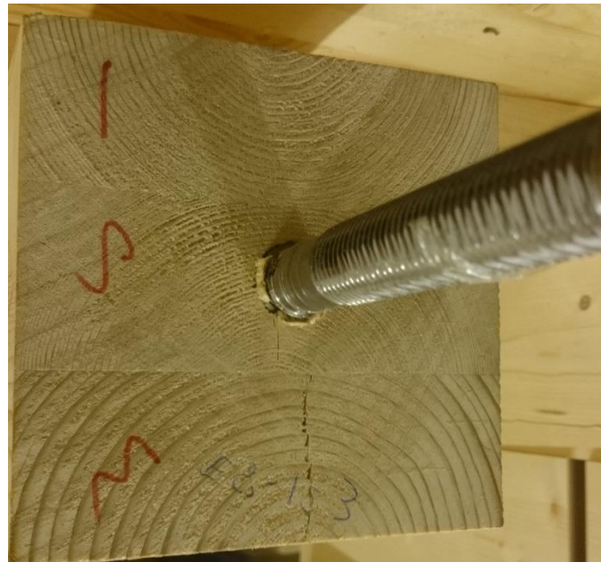
Figure 17 – numbering of specimen, number starts at lamella with annular rings oriented in opposite direction.
