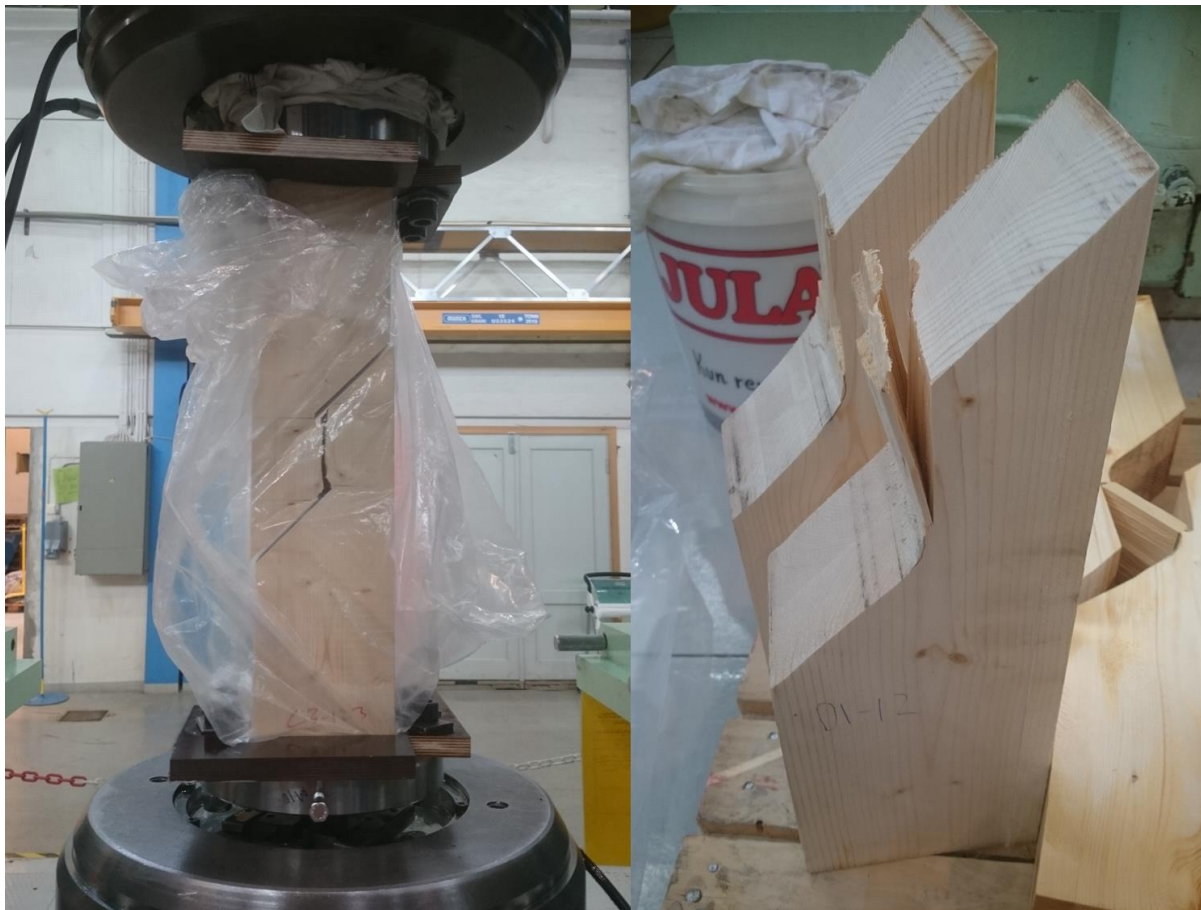
Figure 50-Pictures of fracture patterns in shear
