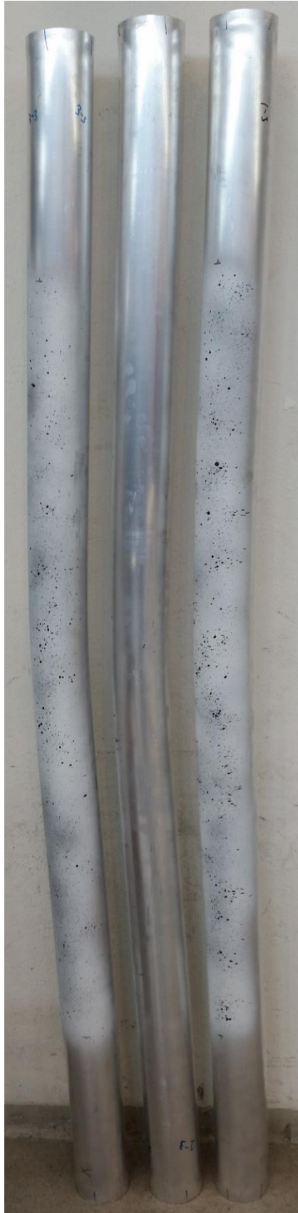
Figure g4 Post-buckling shape specimen 1-2long, 2-2long and 3-2long (A6082D100L2000mm)
