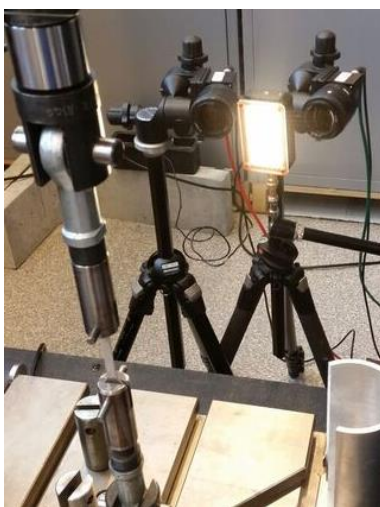
Figure 20 Camera setup to allow usage of DIC technology
