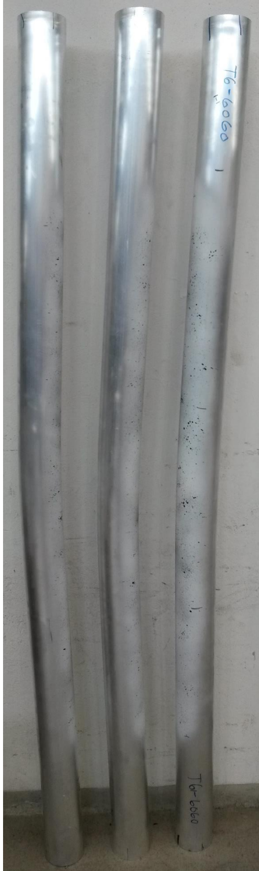
Figure g1 Post-buckling shape specimen 1-1long, 2-3long and 3-3long (A6060D100L2000mm)
