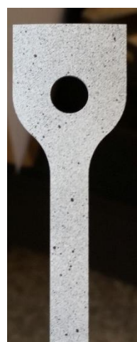
Figure 21 Typical speckled paint applied to the dog bone
