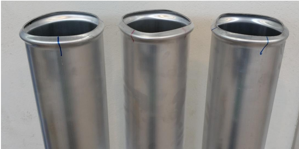
Figure g3 Closeup post-buckling shape for A6060D127L2000mm
