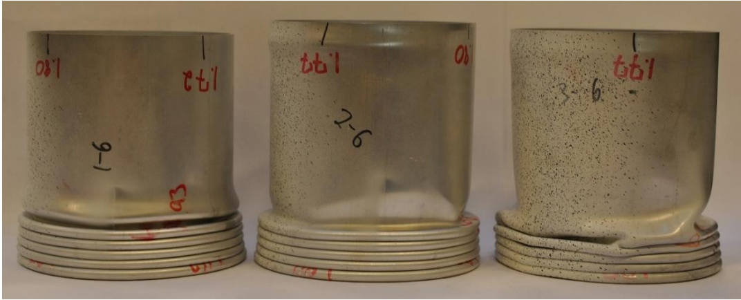
Figure e7 Post-buckling shape specimen 1-6, 2-6 and 3-6 (A6060D127L2D)
