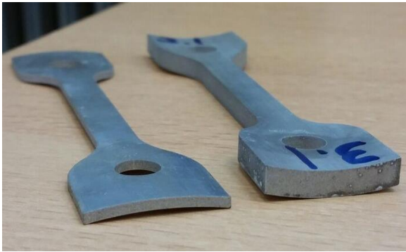
Figure 17 The dog bone specimens were slightly curved.
