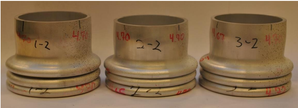
Figure e5 Post-buckling shape specimen 1-2, 2-2 and 3-2 (A6060D100L2D)
