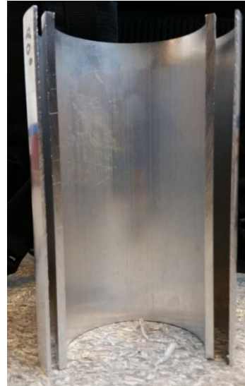
Figure 18 The specimens were cut out of the cylinders
