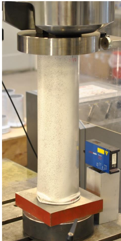
Figure 54 Setup in laboratory during testing with visible speckled paint
