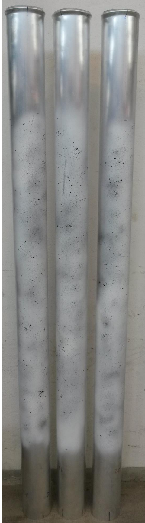
Figure g2 Post-buckling shape specimen 1-2long, 2-2long and 3-2long (A6060D127L2000mm)
