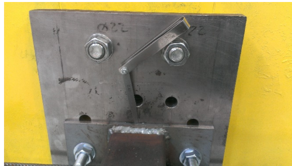
Figure 5.11: Feeler gauge measurement on the gap
