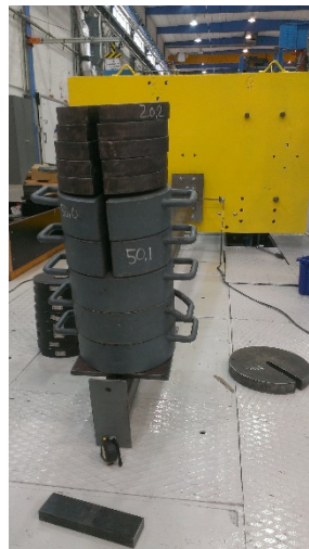
Figure 5.10: Plastic procedure at a weight of 360 kg
