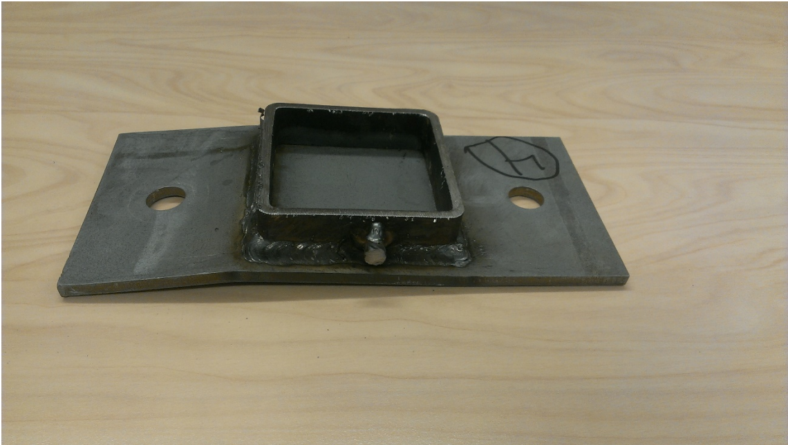
Figure 9.11: Deformation of specimen A about the strong axis
