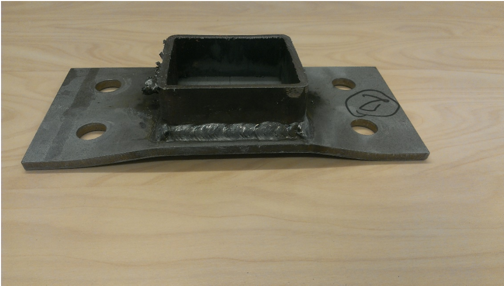
Figure 9.13: Deformation of the specimen B about the weak axis
