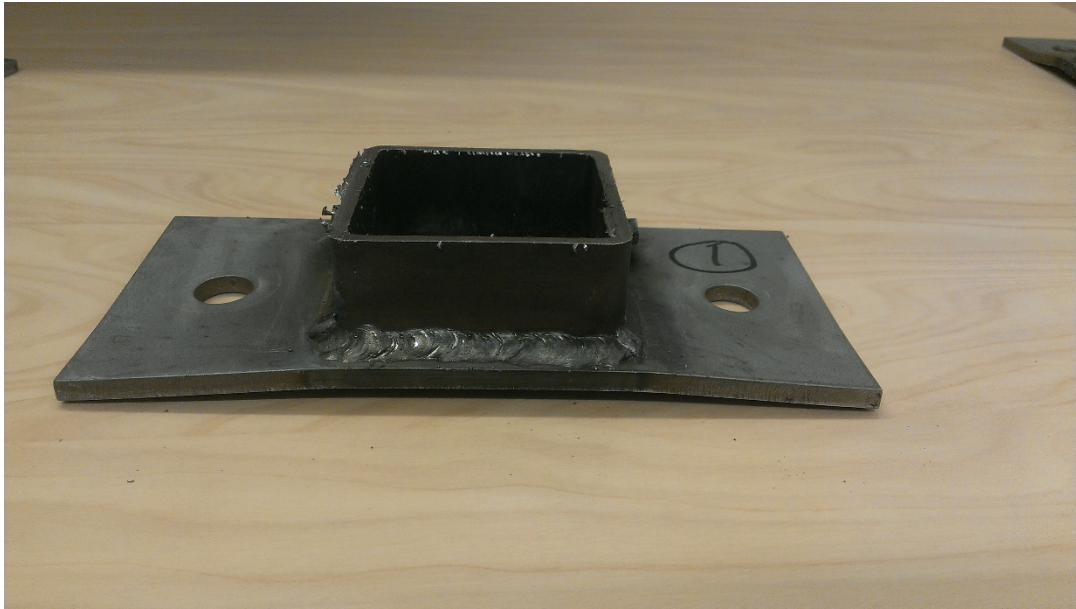
Figure 9.9: Deformation of specimen A about the weak axis
