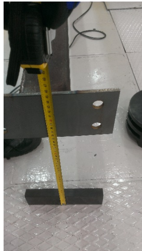
Figure 5.9: Tape measure at the tip of the column
