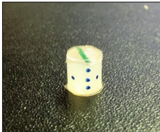
Figure 35: Compression test specimen. The specimen has a diameter and height of 6 mm. The top and bottom surface is layered with tape to reduce friction.
