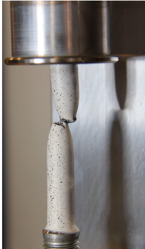
Figure 4.26: Fracture of material test specimen
