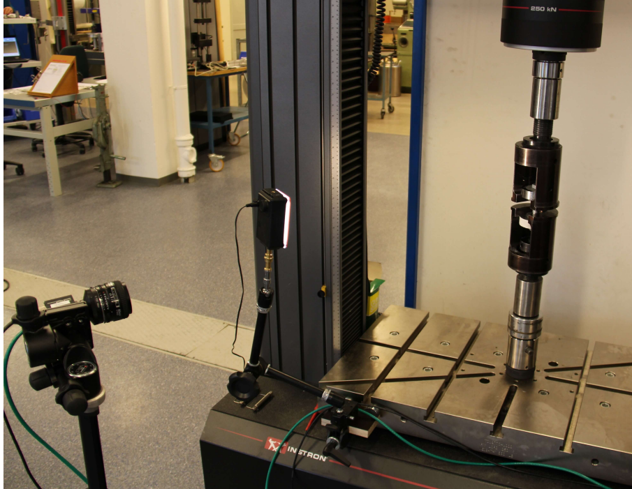
Figure 4.2: Test rig for bolt tests
