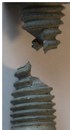
(a) Realistic fracture surface
