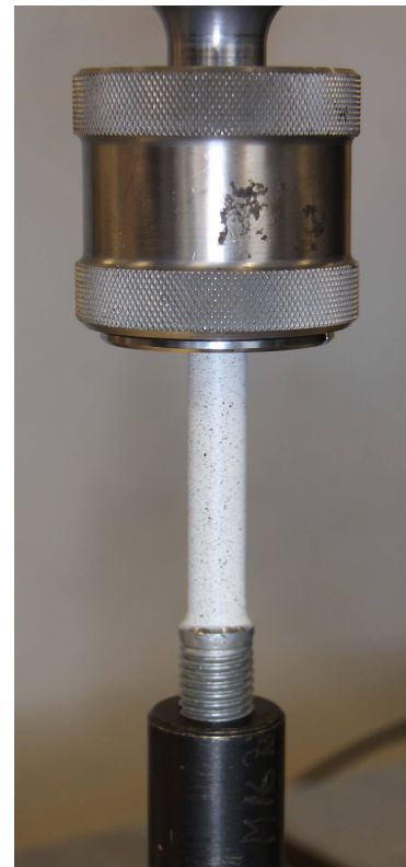
(b) Fastening of test specimen
