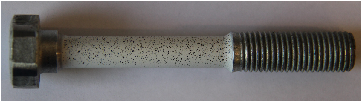
Figure 4.8: Painted material test specimen
