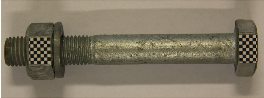
Figure 4.4: Bolt with chess pattern used for DIC analysis
