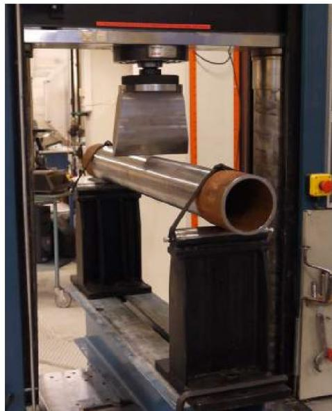
**Figure 1.2:** Setup of quasi-static three-point bending test conducted by M. Kristofferesen [4].
